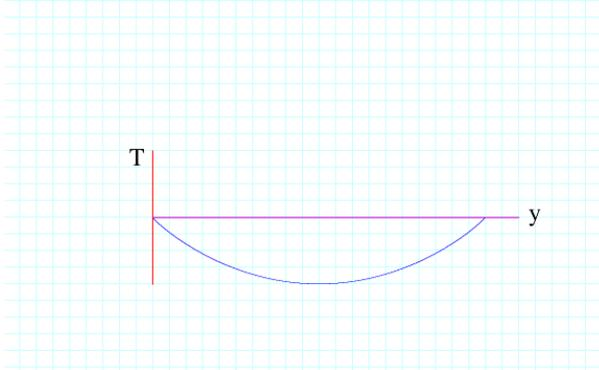
Fig. 9. The temperature profile of linear Couette flow between two walls
