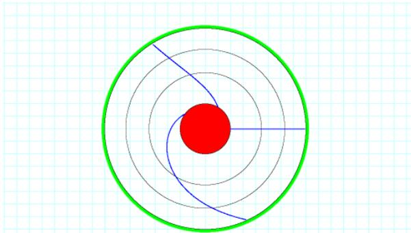
Fig. 3. Snap shot of Couette flow. The horizontal line shows the position of a set of particles at  $t = 0$ ; the two curved lines the same particles at later times. The inner cylinder is rotating clockwise, dragging the fluids along with it.
