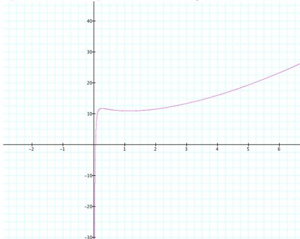
Fig. 5. A temperature profile for cylindrical Couette flow. The small dip for small radius is produced by the  $ab$  term in (6.1). A similar feature has been observed.
