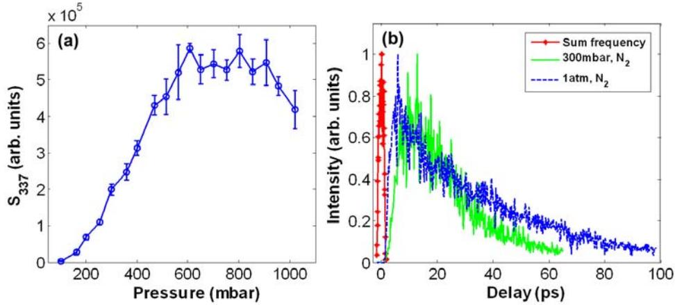
Fig. 4. (a) The intensity of 337-nm nitrogen laser as a function of gas pressures. (b) The temporal evolution of the 337-nm nitrogen laser with the time delay between the pump and probe pulses in the 300-mbar (green solid line) and 1-atm  $N_2$  (blue dashed line).
