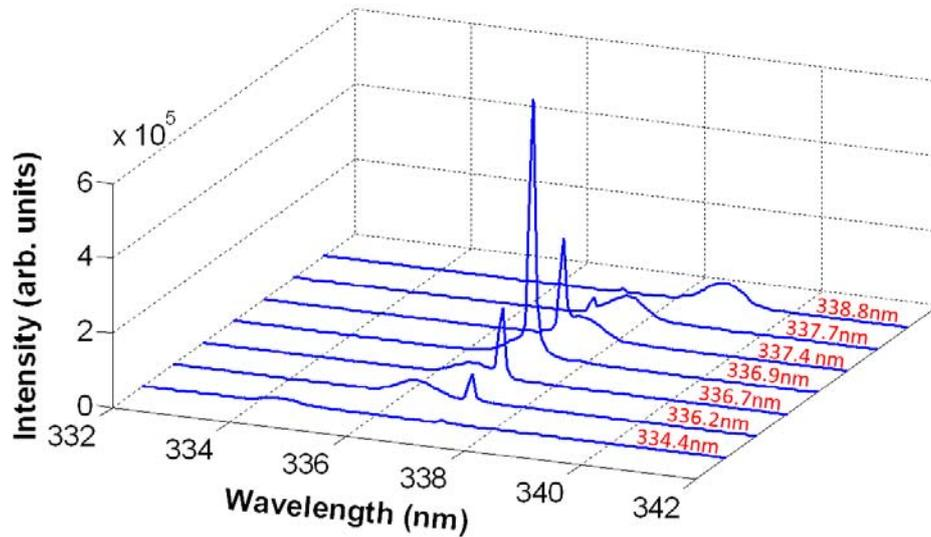
Fig. 3. The signal intensity of 337-nm nitrogen laser as a function of the central wavelengths of the probe pulses, which are indicated on the right side of the corresponding spectra.
