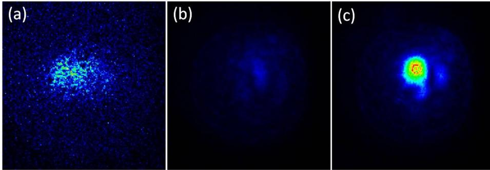
Fig. 4. Spatial profile of the backward ASE (a), the seed pulse (b), and the seeded stimulated radiation (c). The opening angle of each panel is  $24 \text{ mrad} \times 24 \text{ mrad}$ .
