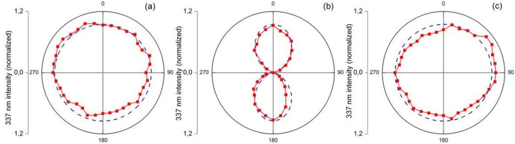
Fig. 3. Polarization properties of the ASE (a), the seeded backward stimulated emission with linearly (b) and circularly (c) polarized seed pulses at 337 nm. The dots present the experimental results and the dashed lines denote the theoretical fitting.
