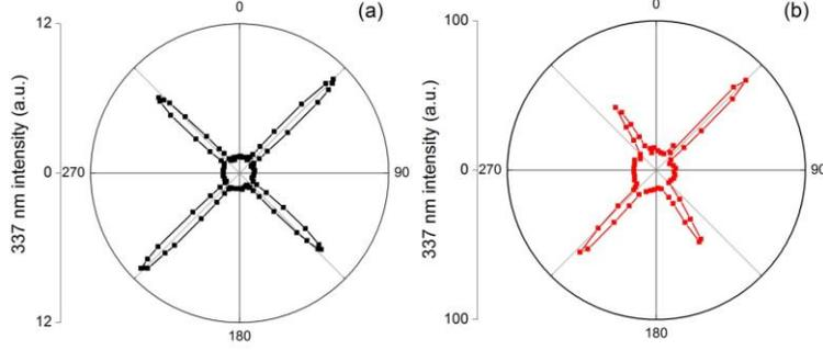
Fig. 5. Dependence of the backward ASE (a) and the seeded backward stimulated radiation (b) as a function of the rotation angle of the quarter-wave plate. The angles  $\phi = 90^\circ \times m$  correspond to linearly polarized laser, with  $m = 0, 1, 2, 3$ . The angles  $\phi = 45^\circ + 90^\circ \times m$  correspond to circularly polarized laser.
