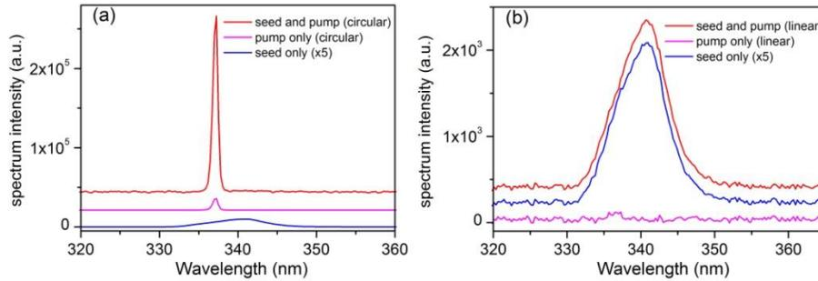
Fig. 2. Spectra of the backward stimulated emission with circularly (a) and linearly (b) polarized pump pulsed at 800 nm. The spectra of the seed pulses and those of the backward emission from just the pump pulses are also presented for comparison.
