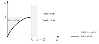
Figure 10. The qualitative behavior of the pendulum for large/small values of torque and damping, as reported in [46, p. 272].
