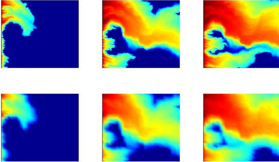
Figure 8: The saturation profile using PG DG-LOD for the pressure equation on the grid  $\mathcal{T}_H$  (bottom) and the reference solution on the grid  $\mathcal{T}_h$  (upper) at time  $T_1 = 0.05$  (left),  $T_2 = 0.25$  (middle), and  $T_3 = 0.45$  (right) using permeability  $K_2$ .
