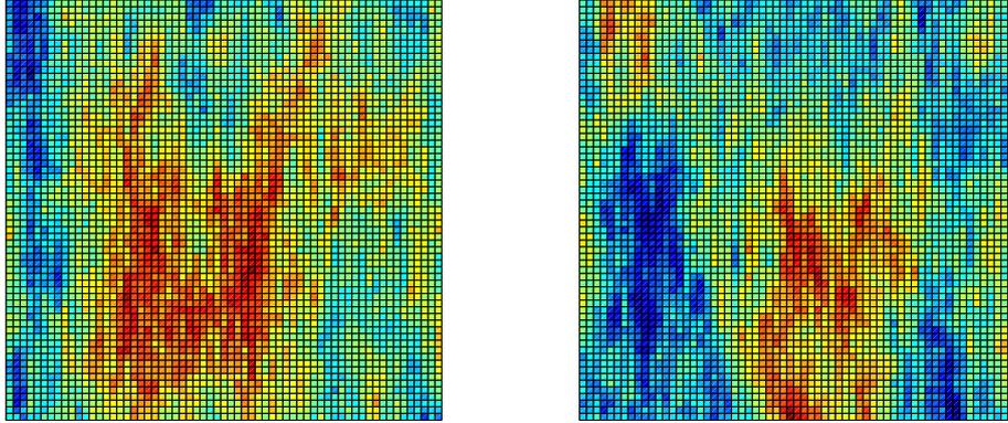
Figure 6: The permeability structure of  $K_i$  in log scale with,  $\beta_0/\alpha_0 \approx 5 \cdot 10^5$  for  $i = 1$  (left) and  $\beta_0/\alpha_0 \approx 4 \cdot 10^5$  for  $i = 2$  (right).
