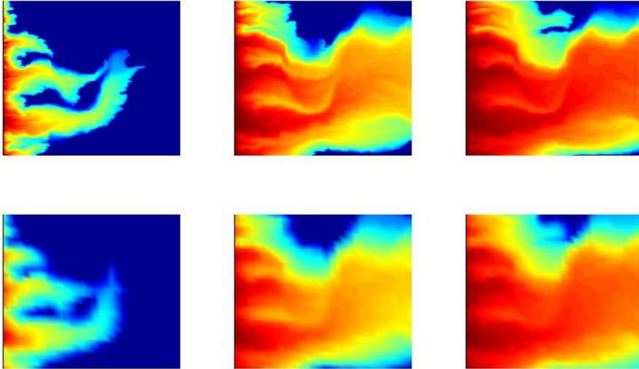
Figure 7: The saturation profile using PG DG-LOD for the pressure equation on the grid  $\mathcal{T}_H$  (bottom) and the reference solution on the grid  $\mathcal{T}_h$  (upper) at time  $T_1 = 0.05$  (left),  $T_2 = 0.25$  (middle), and  $T_3 = 0.45$  (right) using permeability  $K_1$ .
