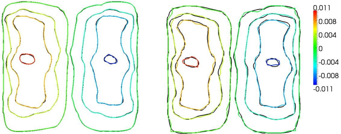
Figure 5: The pictures depict a comparison of isolines. The black lines belong to the reference solution  $u_h$  for  $h = 2^{-8}$ . The colored isolines in the left picture belong to the PG-LOD approximation  $u^{\text{PG-LOD}}$  and match almost perfectly with the one from the reference solution. The right picture shows the coarse part of  $u^{\text{PG-LOD}}$ , i.e.  $P_{L^2}(u^{\text{PG-LOD}})$ . We observe that the isolines still match nicely.
