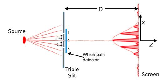
**Fig. 1** A schematic diagram of the 3-slit interference experiment, with a quantum which-path detector.
