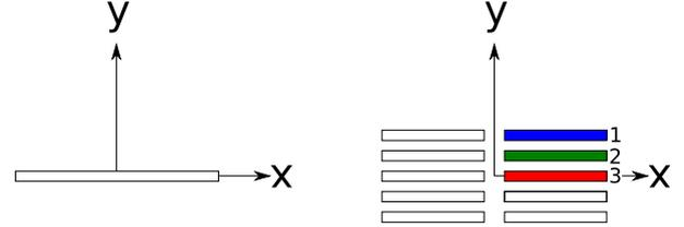
Fig. 1. Schematic illustration of the utilized geometries: cross-section of a single tape (left) and of a Roebel cable (right). All the models are 2-D, so that the current flows perpendicular to the  $x-y$  plane. The colored rectangles represent the tapes along whose width the current profiles are calculated later in the paper.
