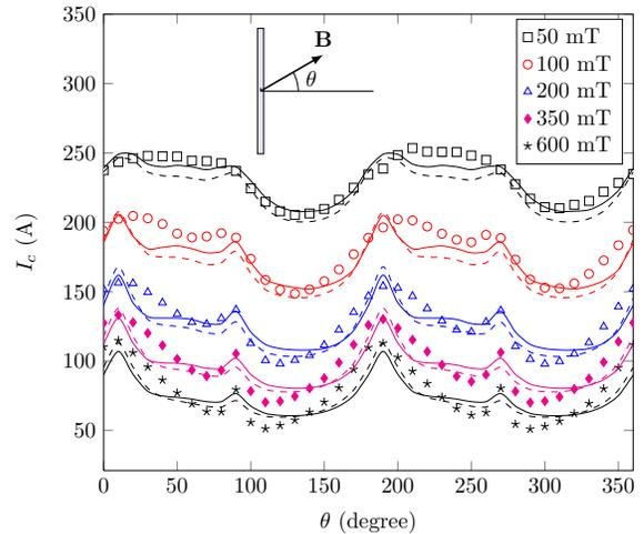
Fig. 7. Comparison of experimental (symbols) and calculated (lines) angular dependence on the applied magnetic field for the coated conductors used to assemble the high-current Roebel cables. The continuous and dashed lines represent the calculated values with the two set of parameters in the  $J_c(B, \theta)$  dependence given in Table III. The self-field critical currents calculated with those two sets are 340 and 339 A, respectively.
