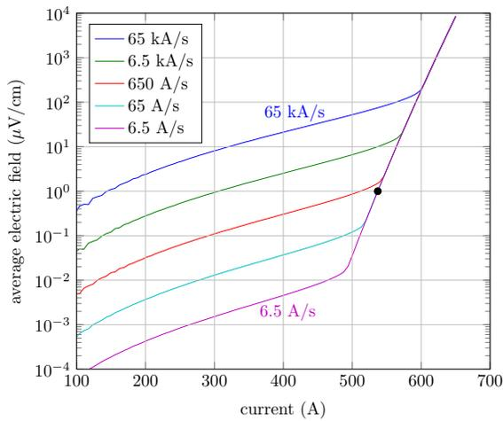
Fig. 9.  $E-I$  characteristics for a Roebel cable calculated with the transient  $H$ -formulation model using current ramps of different speeds. Only the slowest ramps give the correct value of the critical current (537 A, indicated by the black dot), taken when the average field reaches  $1 \mu\text{V}/\text{cm}$ .
