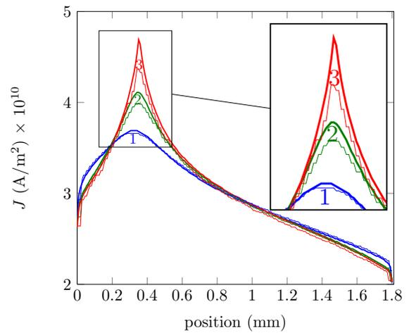
Fig. 10. Comparison of the current density distribution at  $I = I_c$  computed with the static critical state (thick lines) and transient  $H$ -formulation (thin lines) models. The profiles are taken along the width of tapes number 1, 2, 3 of Fig. 1.
