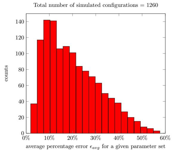
Fig. 4. Statistical distribution of the average percentage of error for all simulated cases with respect to the experimental data.
