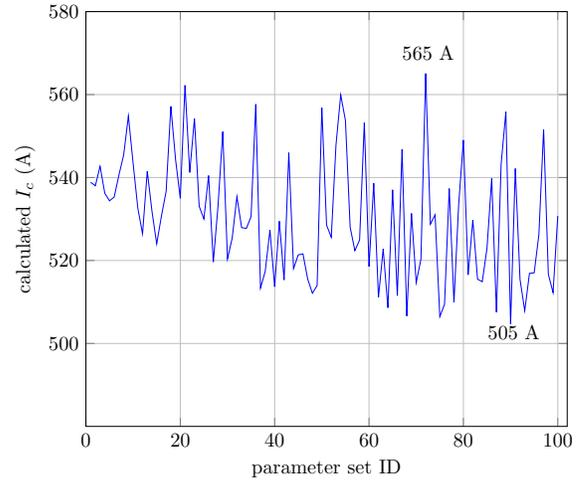
Fig. 5. Critical current of the Roebel cable calculated for the best 100 parameter sets of the  $J_c(B, \theta)$  of a single tape: the highest and lowest value are 565 A and 505 A, respectively.
