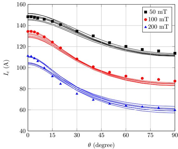
Fig. 3. Calculated angular dependence of the critical current  $I_c$  for the best seven parameter sets (continuous lines) and experimental values (symbols). For the latter, the data of Fig. 2 were averaged over the four quadrants. The self-field calculated  $I_c$  values are given in the last column of Table II.
