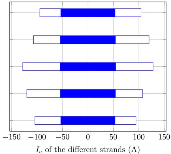
Fig. 6. Calculated critical current in the different strand positions for the low-current (blue bars) and high-current (white bars) Roebel cables. The low-current cable was simulated with the parameter set #1 of Table II. The high-current cable with the set given in the upper part of Table III.
