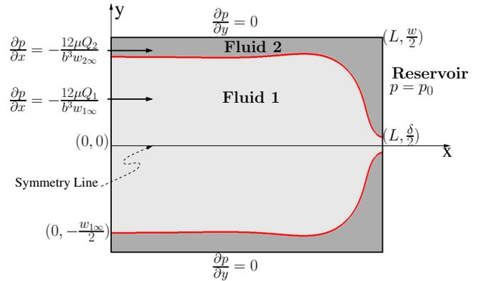
**Fig. 2** Schematic of the flow domain for the Hele-Shaw model and the corresponding boundary conditions. The domain is bounded by walls at  $|y| = w/2$ . At  $x = 0$ , fluid 1 occupies  $|y| \leq w_{1\infty}/2$  and fluid 2 occupies  $w_{1\infty}/2 < |y| \leq w/2$  and  $-w < y < -w_{1\infty}/2$ ;  $w_{2\infty} = w - w_{1\infty}$
