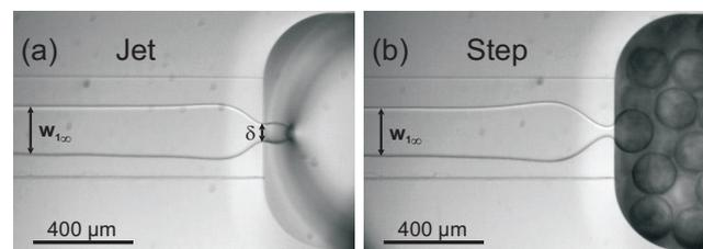
**Fig. 1** Optical micrographs showing two regimes of droplet production. (a) “Jet-emulsification” for large  $Ca$ : Breakup occurs downstream, (b) “Step-emulsification” for low  $Ca$ : Breakup occurs at the step
