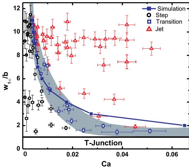
**Fig. 4** Phase diagram demonstrating the transition of jet-regime (red triangles) to step-regime (black circles). Blue open squares denote the transition regime, where droplet production alternates between step- and jet-regime. Blue solid squares indicate the simulation results for  $A = 0.4$ , as discussed in the text. For  $w_{1\infty}/b \leq 1$  no stable filament is formed
