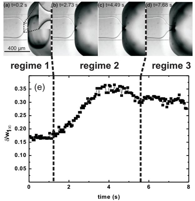
**Fig. 3** Temporal evolution of the tongue in the jet-regime. (a)-(d) Micrographs with the inset showing the interface directly at the step and (e) the shape factor,  $\delta/w_{1\infty}$ , as a function of time;  $Ca = 9.73 \times 10^{-3}$  and  $Q_{1\infty}/Q_{2\infty} = 3$
