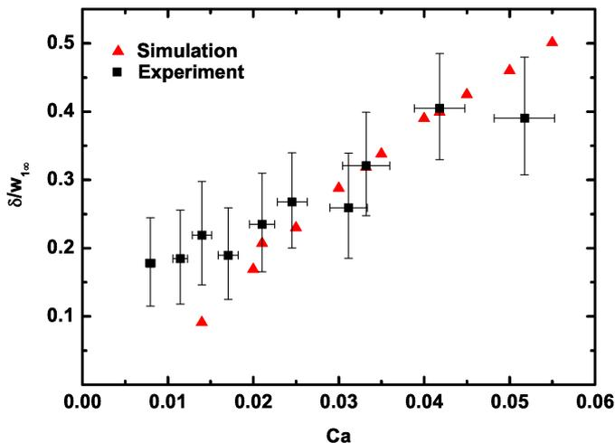
**Fig. 6** Comparison of the experimentally determined shape factor,  $\delta/w_{1\infty}$ , for  $Q_{1\infty}/Q_{2\infty} = 3$  (black squares) and the simulation results (red triangles) for  $Q_{1\infty}/Q_{2\infty} = 2.81$  and  $A = 1$
