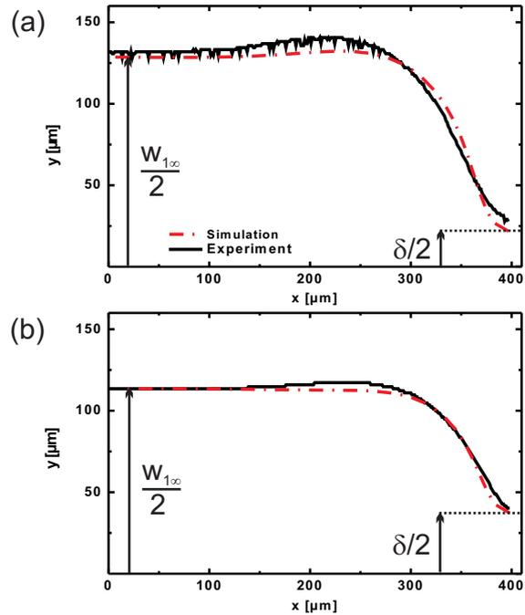
**Fig. 5** Comparison of the tongue profiles in the terrace obtained from experiments (black solid line) and simulations with  $A = 1$  (red dashed line). Both experimental profiles are obtained in the jet-regime. (a)  $Ca = 0.019$  and  $w_{1\infty}/b = 7.97$  and (b)  $Ca = 0.042$  and  $w_{1\infty}/b = 7.44$ . For experiments,  $Q_{1\infty}/Q_{2\infty} = 1.5$ . For simulations,  $Q_{1\infty}/Q_{2\infty} = 1.67$  in (a) and  $Q_{1\infty}/Q_{2\infty} = 1.41$  in (b)
