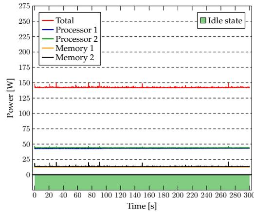
Figure 2: Power of chips and memories on the IBM blade server PS702 during an idle state.
