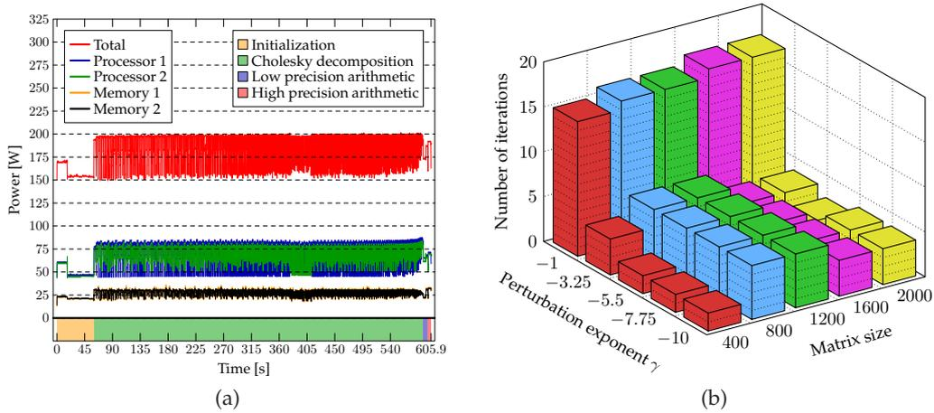
Figure 3: (a) Power diagram on IBM PS702 Blade Server during the solution of a dense linear system with 32 right-hand sides, employing the Cholesky based approach with iterative refinement. In the timeline, each computational phase is displayed with a different color. (b) The number of iterations to solution of a perturbed Cholesky algorithm, for a range of matrix sizes and perturbation exponents.
