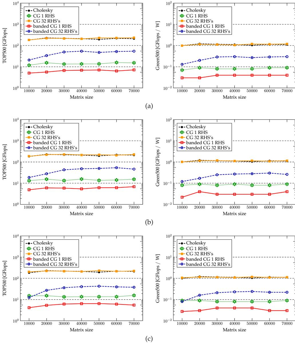
Figure 6: Standard metrics applied to a range of methods for the solution of power model covariance matrices of different size. (a)  $d = 1$ . (b)  $d = 2$ . (c)  $d = 4$ .
