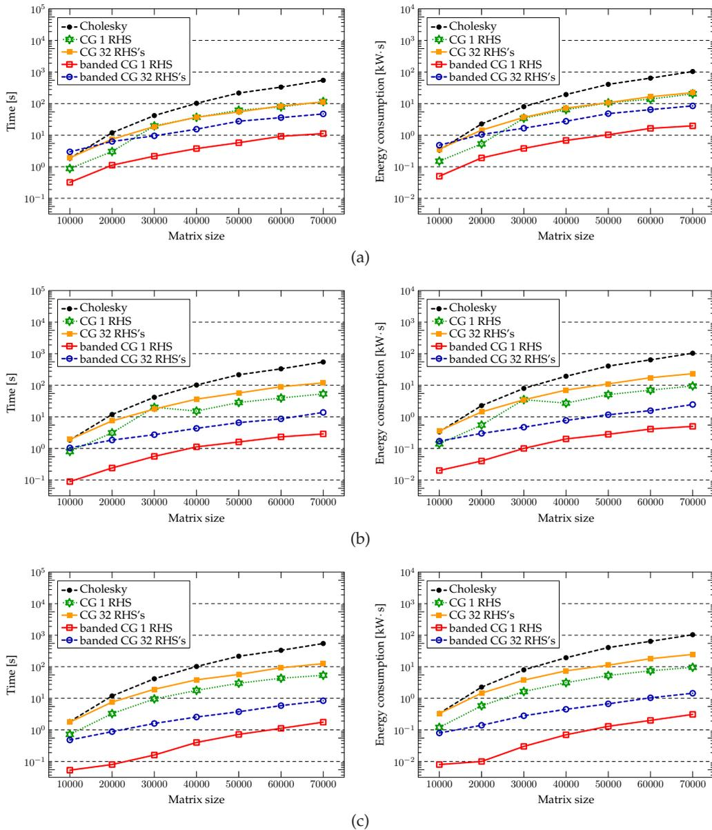
Figure 5: Time and energy comparison between different methods for the solution of power model covariance matrices of different size. (a)  $d = 1$ . (b)  $d = 2$ . (c)  $d = 4$ .
