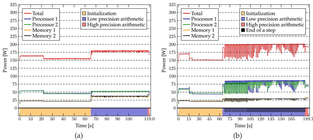
Figure 4: Power diagrams on IBM PS702 Blade Server during the solution of a dense linear system using the conjugate gradient algorithm with iterative refinement. In the timeline, each computational phase is displayed with a different color, while the end of each step is marked by a black line. (a) 1 right-hand side. (b) 32 right-hand sides.
