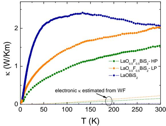
**Figure 4: (color online)** thermal conductivity versus temperature curves of undoped  $\text{LaOBiS}_2$  and doped  $\text{LaO}_{0.5}\text{F}_{0.5}\text{BiS}_2$  polycrystals, prepared either with or without high pressure annealing. Dashed lines indicate the electronic contribution to the thermal conductivity estimated with the Wiedemann-Franz (WF) law.
