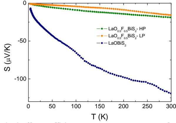
**Figure 3: (color online)** Seebeck effect coefficient versus temperature curves of undoped  $\text{LaOBiS}_2$  and doped  $\text{LaO}_{0.5}\text{F}_{0.5}\text{BiS}_2$  polycrystals, prepared either with or without high pressure annealing.
