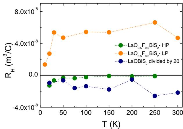
**Figure 2:** (color online) Hall coefficient versus temperature curves of undoped  $\text{LaOBiS}_2$  and doped  $\text{LaO}_{0.5}\text{F}_{0.5}\text{BiS}_2$  polycrystals, prepared either with or without high pressure annealing.
