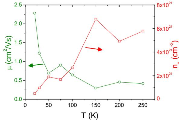
**Figure 5: (color online)** electron charge density and mobility obtained from single band fitting of  $\rho$  and  $R_H$  data of doped LaO<sub>0.5</sub>F<sub>0.5</sub>BiS<sub>2</sub>\_HP sample, prepared with high pressure annealing.
