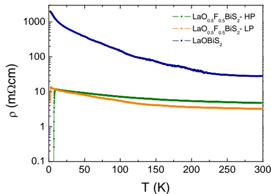
**Figure 1: (color online)** resistivity versus temperature curves of undoped  $\text{LaOBiS}_2$  and doped  $\text{LaO}_{0.5}\text{F}_{0.5}\text{BiS}_2$  polycrystals, prepared either with or without high pressure annealing.
