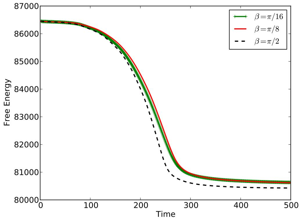
Figure 13: Effect of rotation angle on the crystallites. The plotted solutions use a time step size  $\Delta t = 0.5$ , a stabilization parameter  $\alpha_n = 0.5$ , and  $[150]^3$  linear elements. Three different rotation angles  $\beta$  are considered.
