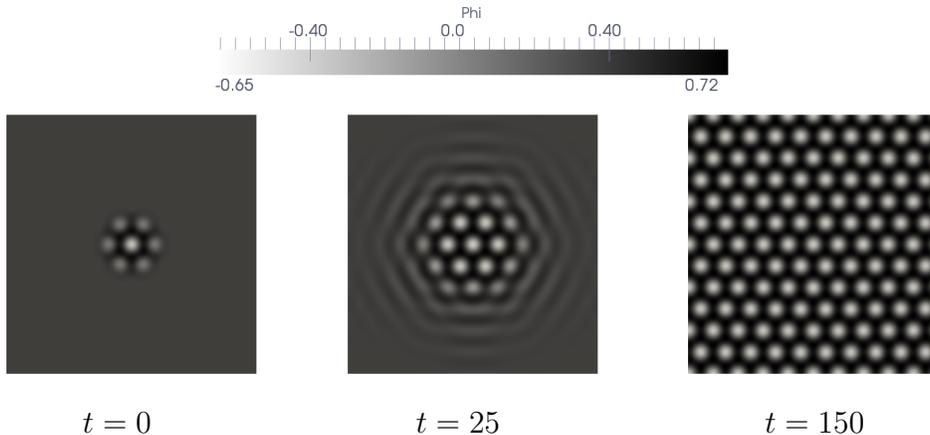
Figure 1: Snapshots of the approximate dimensionless atomistic density field showing its evolution throughout the simulation, which was run using a computational mesh composed of  $256 \times 266$   $C^0$  linear elements, with a time step size of 1.0.
