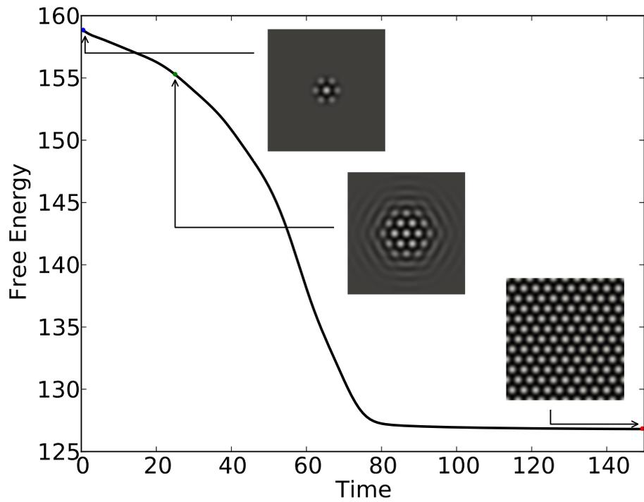
Figure 2: Free energy evolution. The free energy is monotonically decreasing throughout the simulation, which was run using a computational mesh composed of  $256 \times 266$   $\mathcal{C}^0$  linear elements. A time step size of 1 was used, with an  $\alpha_n$  value of 0.25.
