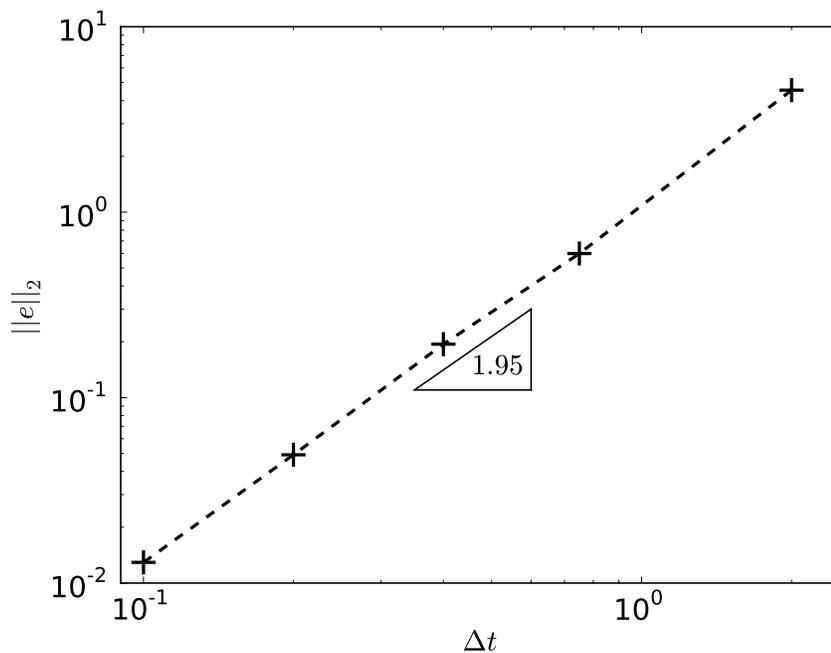
Figure 5: Log of  $\mathcal{L}^2$ -norm of the error at time  $T = 150$  versus the log of time step size  $\Delta t$ . The value of the slope confirms the method is second-order accurate in time. The mesh used was made up of  $[128 \times 133]$  quadratic  $\mathcal{C}^0$  elements, such that the spatial error could be considered negligible in the simulations. The parameter  $\alpha_n$  was given a value equal to 0.25, which complies with the bound presented in section 3.1.3 for this problem.
