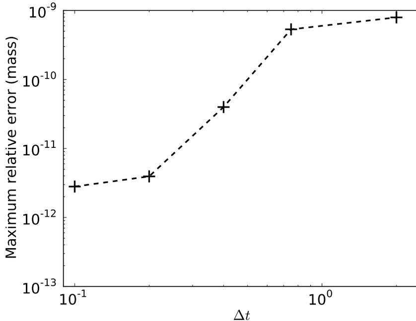
Figure 6: Mass conservation. The maximum relative error over the entire evolution of the system remained below  $10^{-9}$  for the simulations considered in this work. The mesh used was made up of  $[128 \times 133]$  quadratic  $\mathcal{C}^0$  elements, such that the spatial error could be considered negligible in the simulations. The parameter  $\alpha_n$  was given a value equal to 0.25, which complies with the bound presented in section 3.1.3 for this problem.
