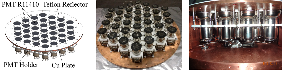
FIG. 7: Left panel: Mechanical design of the bottom PMT array and the teflon reflectors. Center panel: Photograph showing all 37 R11410 PMTs installed on the copper plate of the bottom PMT array. Right panel: Photograph showing the bottom PMTs with the copper filler and how they are connected to the bottom feedthroughs.
