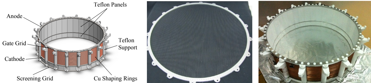
FIG. 5: Left panel: Mechanical design of the field cage showing the teflon panels and supports, three electrodes and the field shaping rings. Center panel: Photograph of the wire electrode for the gate grid, the cathode and the screening electrodes. Right panel: Photograph showing the anode mesh is fixed above the grid ring with a teflon ring in between.
