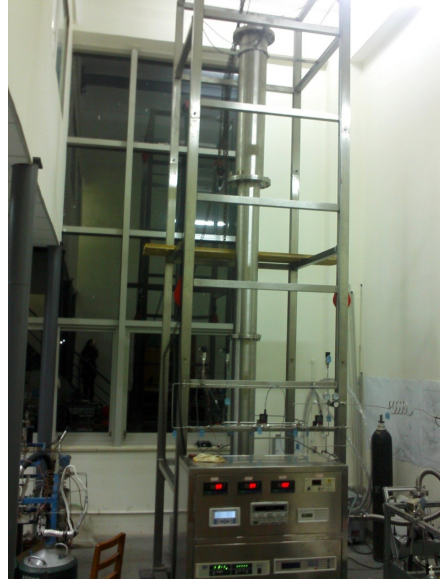
FIG. 19: Left panel: Schematic overview of the technological process of the cryogenic distillation system, 1–Getter, 2–Heat exchanger, 3–Cryo-cooler 1, 4–Cryo-cooler 2, 5–Condenser, 6–Distillation column, 7–Liquid meter, 8–Re-boiler, 9–Vacuum jacket. Right panel: Photograph of the actual distillation system.
