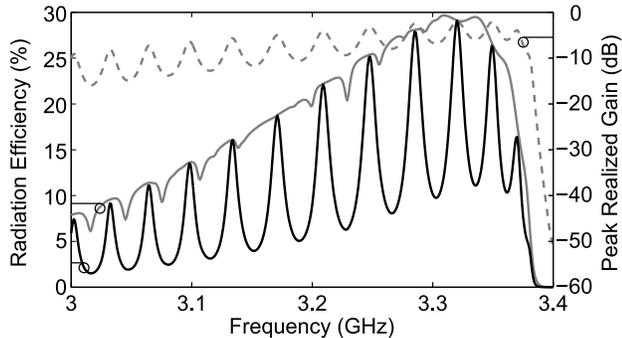
Fig. 7. Radiation efficiencies for the shielded-loop-excited OEWG, defined by  $\eta_{r,i} = P_{rad}/P_{inc}$  (solid black curve) and  $\eta_{r,a} = P_{rad}/P_{acc}$  (solid grey curve). The peak realized gain (dashed grey curve) is also shown.
