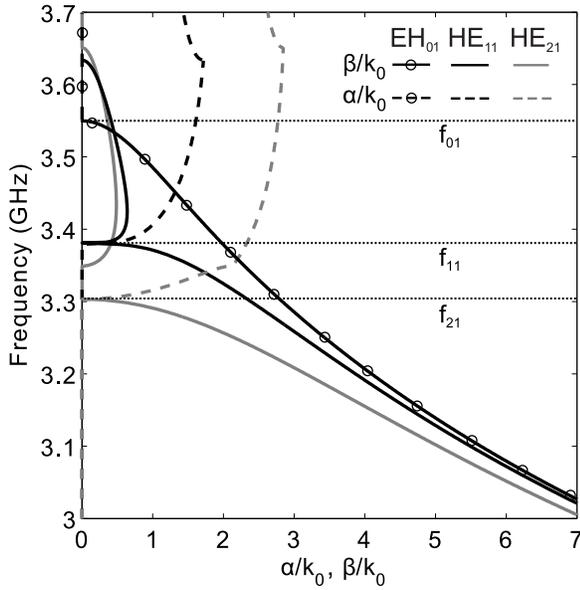
Fig. 2. Dispersion of  $\alpha/k_0$  (dashed curves) and  $\beta/k_0$  (solid curves) for the isotropic metamaterial-lined waveguide's  $HE_{11}$  (black curves),  $HE_{21}$  (grey curves), and  $EH_{01}$  (black circle markers) modes.
