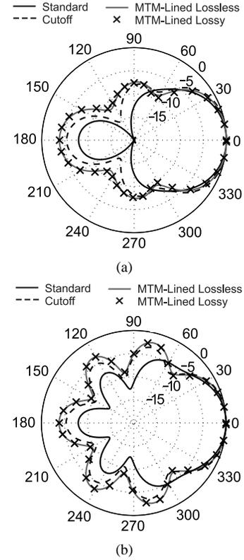
Fig. 5. Comparing normalized (a) H-plane and (b) E-plane directivity patterns of the OEVG obtained from simulations of the ‘Standard’, ‘Cutoff’, and ‘MTM-Lined’ (Lossless and Lossy) cases. All data presented at  $f = 3.381\text{GHz}$ .
