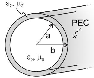
Fig. 1. A PEC circular waveguide consisting of two concentric dielectric regions: an inner vacuum region of radius  $a$  and an outer dielectric region of thickness  $t = b - a$  described by permittivity and permeability  $\epsilon_2$  and  $\mu_2$ .
