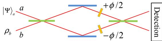
FIG. 1. (Color online) Schematic diagram of a balanced MZI, which is composed of two 50:50 beam splitters (shown in green) and two phase shifters (orange). The input state of the two ports is  $|\psi\rangle_a \langle\psi| \otimes \rho_b$ , where  $|\psi\rangle_a$  is an arbitrary pure state and  $\rho_b$  is a squeezed thermal state.
