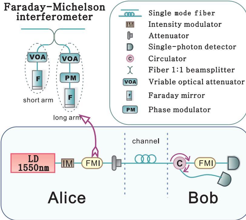
FIG. 1: (color online). The experimental setup of the reference-frame-independent quantum key distribution system with decoy states. Channel attenuation is  $0.20\text{dB}/\text{km}$ . The arm-length difference of the FMI is  $2\text{m}$ .
