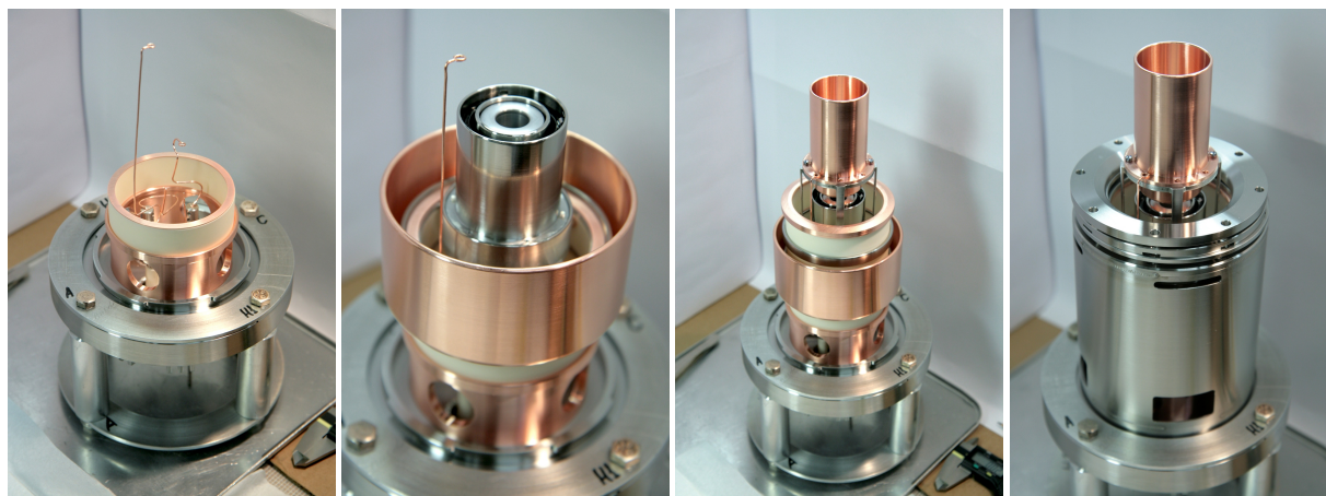
Figure 9. Assembly of the prototype (1-inch) hollow electron gun. The first photograph shows the base flange with electrical connections. In the second photo, one can see the hollow cathode with convex surface and the rim of the control electrode; both are surrounded by cylindrical heat shields. The mounting of the copper anode is shown in the third picture. The last picture shows the complete assembly.
