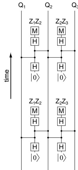
FIG. 1. Two measurement qubits (repeatedly initialized to  $|0\rangle$ ) interleaved between the 3 data qubits ( $Q_1 Q_2 Q_3$ ) of a distance 3 repetition code. Two cycles of measuring  $Z_1 Z_2$  and  $Z_2 Z_3$  are shown.
