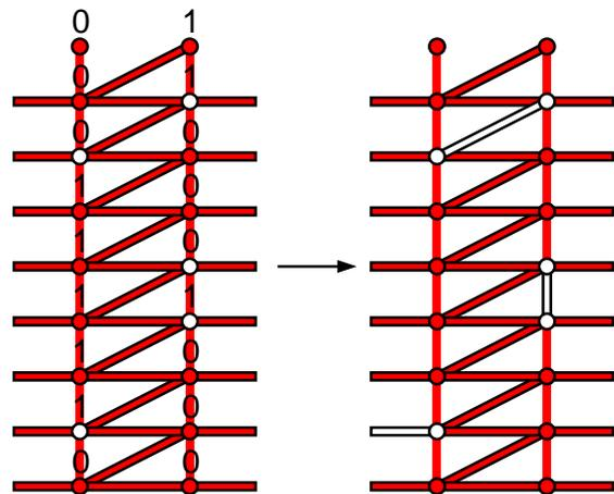
FIG. 4. (left) Pattern of detection events (white circles). (right) Most probable pattern of errors leading to the observed detection events (white lines).
