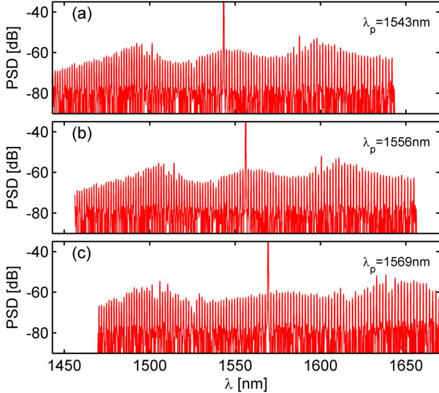
Fig. 4. Microring output spectrum recorded with the OSA for a pump power of  $\sim 30$  mW. (a) pump oscillating at 1543 nm (b) pump oscillating at 1556 nm (c) pump oscillating at 1569 nm.
