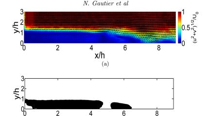
Figure 2: (a) Instantaneous velocity amplitude snapshot. (b) Corresponding instantaneous recirculation area shown in black.
