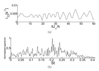
Figure 10: (a)  $\lambda_{Ci}(t)$  signal over 60 seconds, uncontrolled flow. (b) Normalized frequency spectrum showing a peak at 0.97 Hz.
