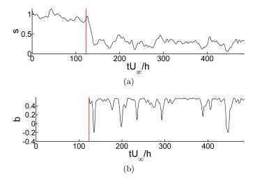
Figure 8: (a) System response s to the control law, the vertical line shows when control starts. (b) Corresponding actuation b.
