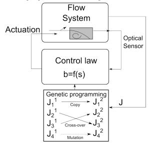
Figure 3: Control loop featuring genetic programming. Control laws b(s) are evaluated by the flow system. This is done over several generations of individuals. New generations are generated by replication, cross-over and mutation  $J_i^n$  refers to the  $i^{th}$  individual of generation n.
