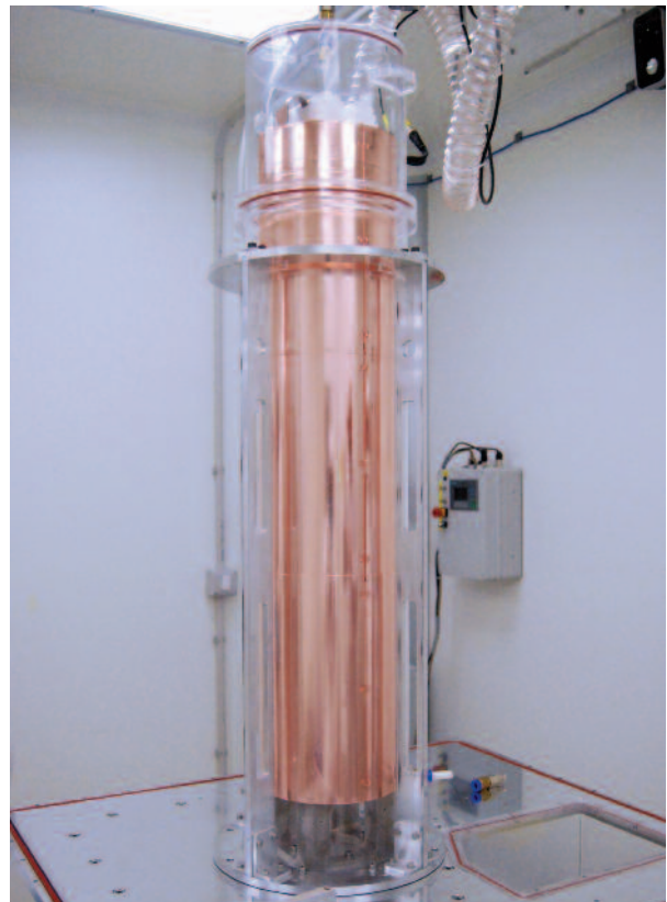
Figure 29: The CUORE-0 tower within the storage box ready to exit the Cuore Tower Assembly Line.
