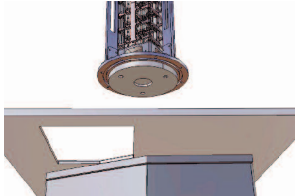
Figure 21: The tower leaving the garage inside the storage box. The same plate the detector has been assembled on provides the bottom closing of the canister.
