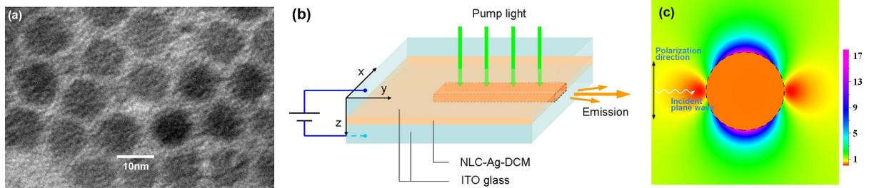
Figure 1: (a) The TEM image shows the morphology and size of silver nanoparticles. (b) Schematic illustration of the configuration of NLC-Ag-DCM sample and the arrangement of excitation-detection. (c) Energy density distribution of a particle plasmon-polariton mode excited by incident photons at  $610\ \text{nm}$ . The dashed black circle labels the particle surface.
