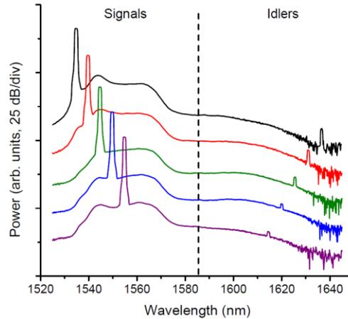
Fig. 13. (Color online) Output spectra for type-I phase matched DFG in a DD-QPM waveguide with different input wavelengths. Reproduced from [100].
