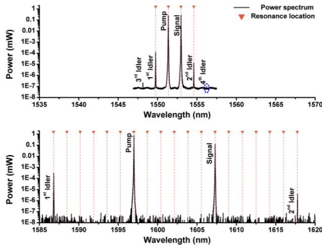
Fig. 16. (Color online) FWM experimental results for two different excitation conditions; dashed lines correspond to resonant frequencies. (upper) The pump and signal lasers are tuned to adjacent resonances and
