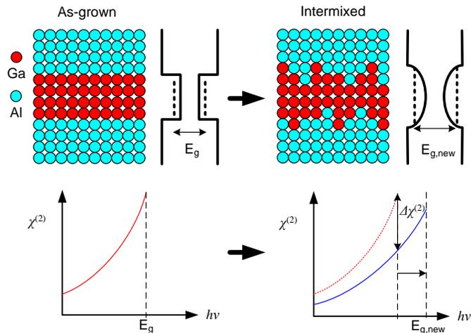
Fig. 5. (Color online) Quantum well intermixing process and the effect on the nonlinear susceptibility.
