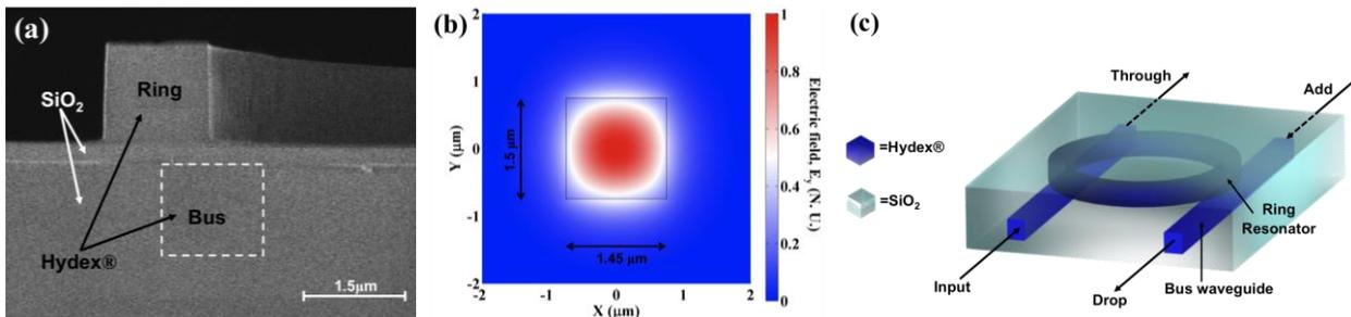
Fig. 3. (Color online) Cross-sectional view of the Hydex® waveguide showing (a) the geometry (picture of the device prior to final SiO<sub>2</sub> deposition to bury the waveguide) and (b) the distribution of the electric field of the fundamental mode. (c) Schematic of the vertically coupled microring resonator.
