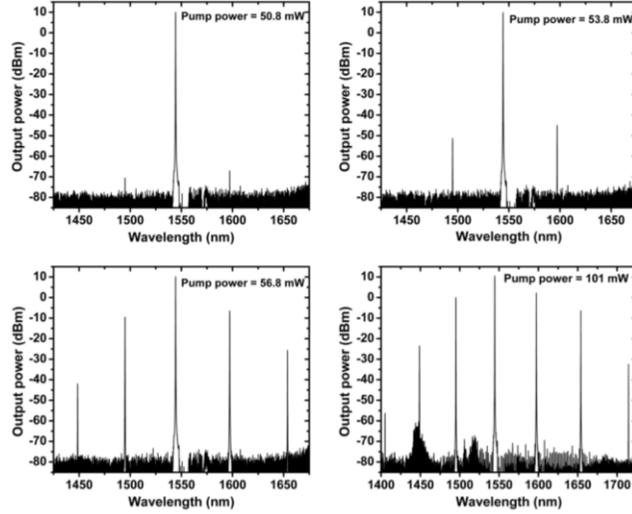
Fig. 18. Experimentally obtained parametric oscillation in the Hydex® microring resonator as a function of the pump ( $\lambda_p = 1544.15$  nm) power. At threshold ( $P_p \sim 54$  mW) we found that a pair of idlers ( $\lambda_s = 1596.98$  nm,  $\lambda_i = 1494.70$  nm) that grow out of noise with an exponential dependence on the pump power is generated. Cascaded FWM can also be observed above threshold, creating another pair of idlers ( $\sim 1448$  nm and  $\sim 1654$  nm).
