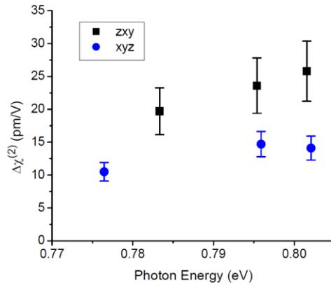
Fig. 12. (Color online) Modulation in  $\chi^{(2)}$  between as-grown and intermixed AlGaAs/GaAs superlattices.
