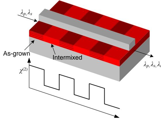
Fig. 6. (Color online) A domain-disordered quasi-phase matching waveguide. As-grown regions retain a large nonlinearity while intermixed regions have a suppressed nonlinearity. Image source: [78].
