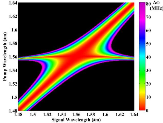
Fig. 15. (Color online) Frequency mismatch in the Hydex® high  $Q$  ring resonator. The color intensity plot represents the net frequency mismatch as a function of the excited pump and signal frequencies (resonances). The region where the frequency mismatch is too large to observe tangible FWM is represented in black. Note that we interpolated the data between resonances for aesthetics and to add clarity in reading the figure.
