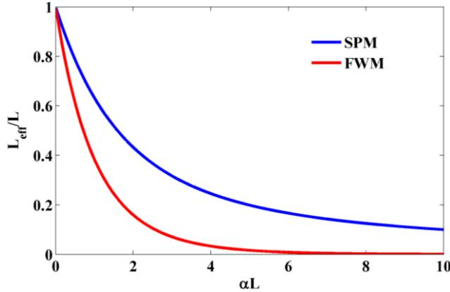
Fig. 2. (Color online) Ratio of the effective nonlinear length  $L_{\text{eff}}$  to the total propagation length  $L$  as a function of the linear losses. The blue curve is for the nonlinear phase accumulated for SPM, whereas the red curve is for wavelength conversion using FWM.
