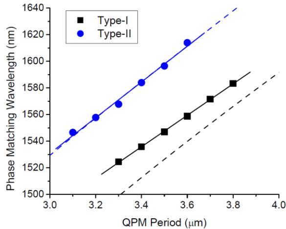
Fig. 11. (Color online) Phase matching wavelengths for SHG in DD-QPM waveguides for different grating periods in both type-I and type-II polarization configurations. Measured data (symbols) and fit trends (solid lines) are shown alongside with the predicted phase matching wavelengths (dashed lines). Image source: [100].
