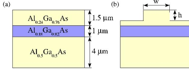
Fig. 4. (Color online) (a) The designed AlGaAs wafer composition and (b) the schematic of a strip-loaded waveguide studied in our experiments:  $w = 2\text{-}3\ \mu\text{m}$ ,  $h = 1.0\text{-}1.2\ \mu\text{m}$ . Image source: [47].
