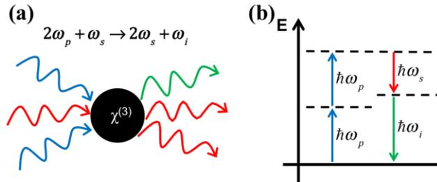
Fig. 1. (Color online) Schematic of the quantum interaction between incident and outgoing photons within the propagating nonlinear medium for a degenerate FWM process. (b) Energy diagram for degenerate FWM where the dashed lines represent virtual levels.
