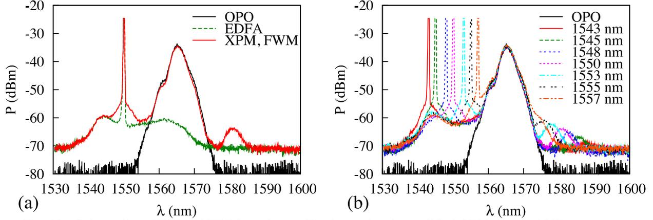
Fig. 10. (Color online) XPM and FWM results. (a) The input signal (amplified CW laser at  $\sim 1547$ nm), green curve, broadens in frequency due to the XPM (red curve) caused by the strong input pump (centered at 1565nm, black curve). FWM is also observed at  $\sim 1580$ nm (red curve). (b) Wavelength tunability of the FWM process, obtained by varying the input signal frequency. Image source: [47].
