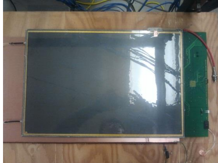
Figure 8. Photograph of a 1-glass RPC. The readout pads can be seen through the resistive paint of the glass plate.
