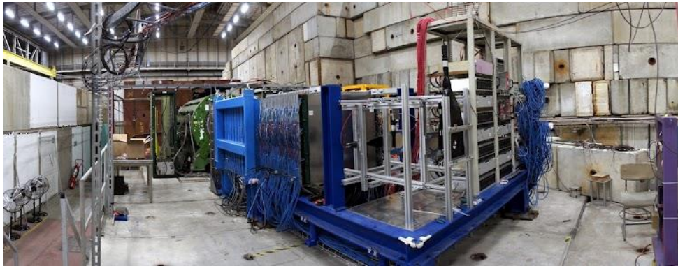
Figure 1. Photograph of the DHCAL main stack and tail catcher, as configured for the CERN PS and SPS test beams
