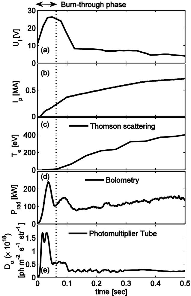
**Figure 1** Typical experimental data during the plasma burn-through phase measured in JET (#77210); (a) Toroidal loop voltage  $U_l$  (Note, at JET  $E_l \sim U_l/20\text{m}$ ), (b) Plasma current  $I_p$ , (c) Electron temperature  $T_e$  (Thomson scattering), (d) Radiated power  $P_{\text{rad}}$  (Bolometry), (e) D alpha emission (Photomultiplier tube).
