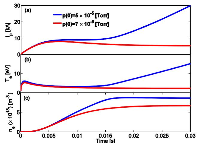
**Figure 4** Typical DYON simulation results for a pure D plasma in JET ( $R=3\text{m}$  and  $a=0.5\text{m}$ ); (a) plasma current, (b) electron temperature, and (c) electron density. Under the same toroidal loop voltage 20 V, different prefill gas pressures are given;  $p(0)=5 \times 10^{-5}$  Torr (blue) and  $7 \times 10^{-5}$  Torr (red).
