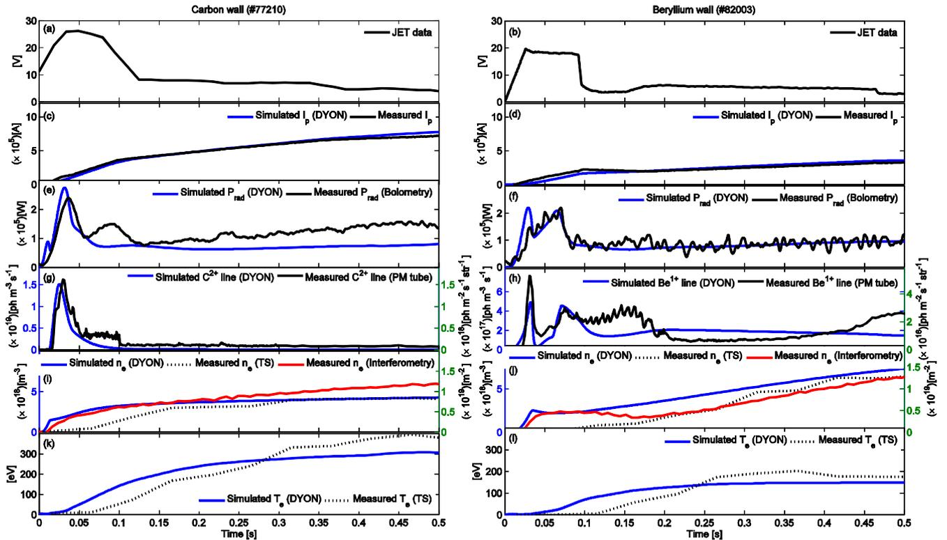
**Figure 6** Comparison of DYON simulation results and JET experiments with the C wall (#77210) [1] and the Be wall (#82003) [2]. (a)(b) toroidal loop voltage, (c)(d) plasma current, (e)(f) total radiation power, (g)(h) photon emission (C2+ and Be1+), (i)(j) electron density, (k)(l) electron temperature. (TS is Thomson Scattering.)
