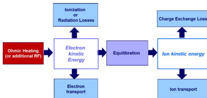
**Figure 2** Energy balance in a plasma during the plasma burn-through phase.
