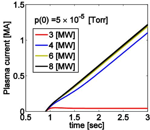
**Figure 10** Simulated plasma current in RF-assisted plasma burn-through simulations for ITER. With the same prefill gas pressure ( $5 \times 10^{-5}$  Torr), the RF power is scanned.
