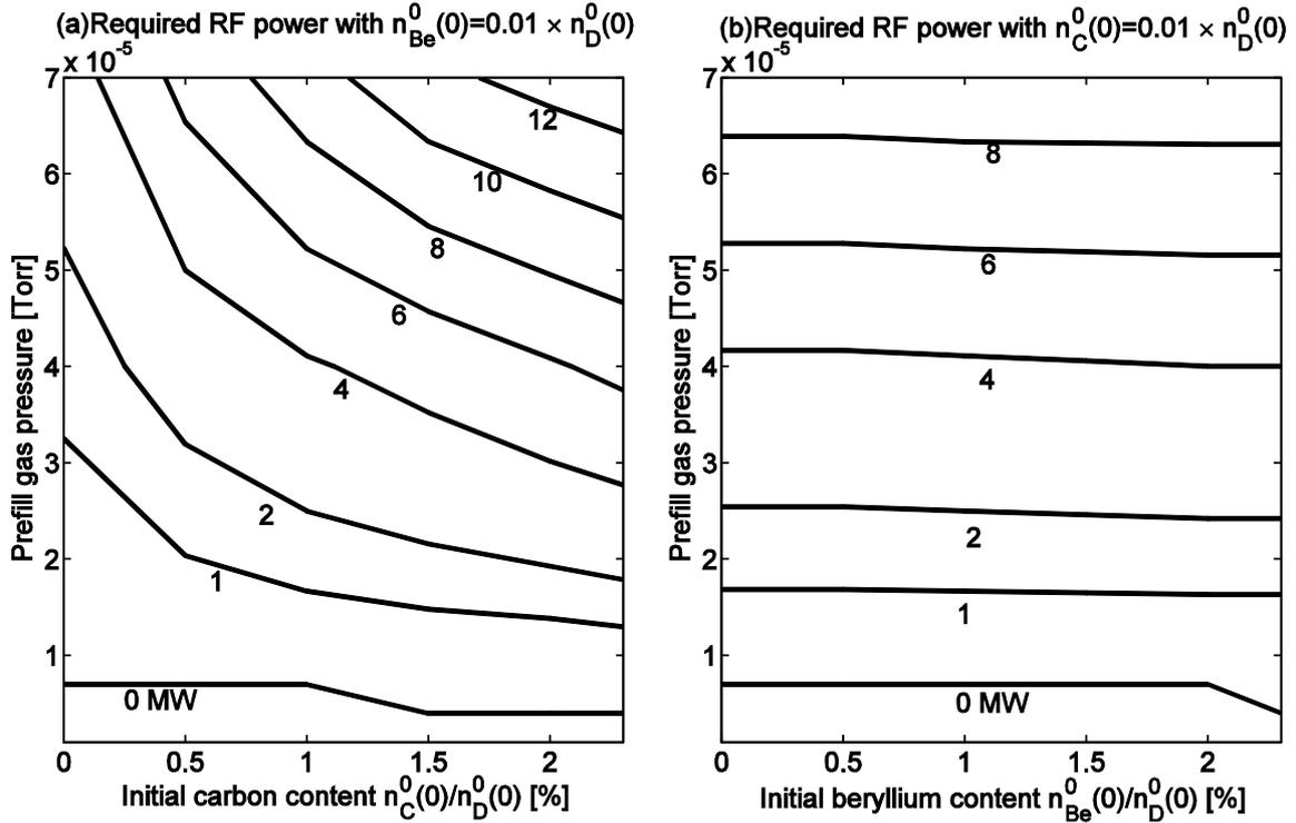
**Figure 12** Estimation of the required RF power using the DYON simulations for successful plasma burn-through in ITER. (a) initial Be content 1% of  $n_D(0)$  (b) initial C content 1% of  $n_D(0)$ .
