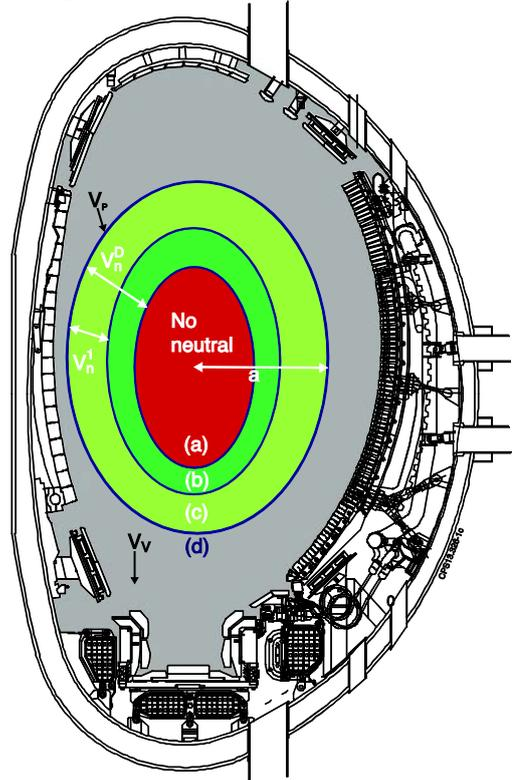
**Figure 5** Ionization shell model.  $V_p (= (a) + (b) + (c))$  is a plasma volume, and  $V_v (= (a) + (b) + (c) + (d))$  is the total vessel volume. Since there are no neutrals in (a), the total neutral volume is  $(b) + (c) + (d)$ .  $V_n^D$  and  $V_n^I$  are the neutral volumes of Deuterium ( $= (b) + (c)$ ) and Impurity ( $= (c)$ ) within the plasma volume  $V_p$ , respectively.
