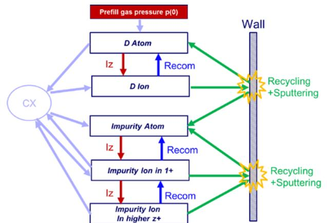
**Figure 3** Particle balance in a plasma during the plasma burn-through phase. CX is charge exchange reaction between D atoms and impurity ions, Iz is impact ionization by free electrons, Recom is Recombination reaction. Wall is the surrounding plasma facing component; in this study the wall material is carbon or beryllium.
