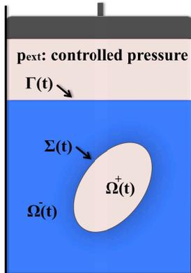
Figure 1. The two phase system under pressure control.
