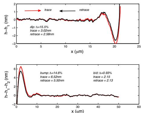
FIG. S2: Average of several tens of scan lines around the dip (top) and bump (bottom), from raw AFM “trace” and “retrace” scans.
