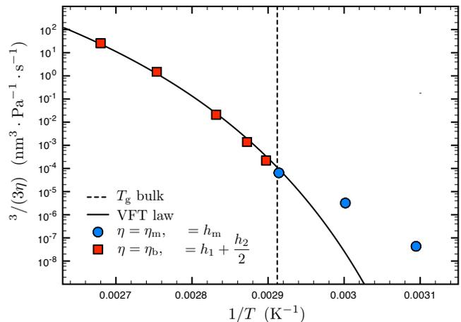
FIG. 5: Fig. 5. Temperature dependence of the mobility. This figure is made of two subplots representing  $h_1 = h_2 = 90 \text{ nm}$  samples. The mobility  $H^3/(3\eta)$  is determined by a fit to either the analytical GTFE solution (blue circles) or the numerical TFE solution (red squares), with  $\eta$  and  $H$  as defined in the legend.
