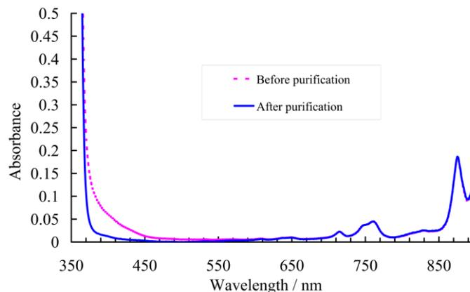
Figure 6. Absorption spectra of LAB containing 10 g/L PPO before and after purification.
