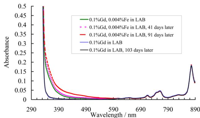
Figure 3. Comparison of absorption spectra of 0.1% Gd-LAB with or without Fe at various times after preparation.
