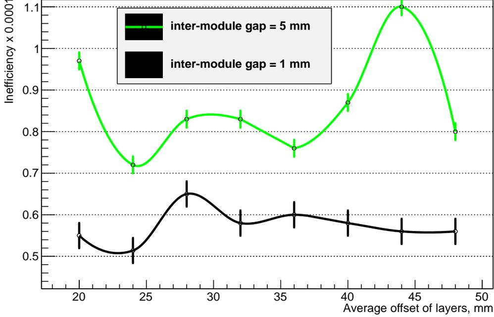
Figure 8. The muon registration inefficiency in the region of the muon-stopping target for two inter-module gaps for the first configuration described in the beginning of the section 2. The gap between the layers is taken to be 3 mm. Notice that the offset of the second layer is a half of the *average offset*.
