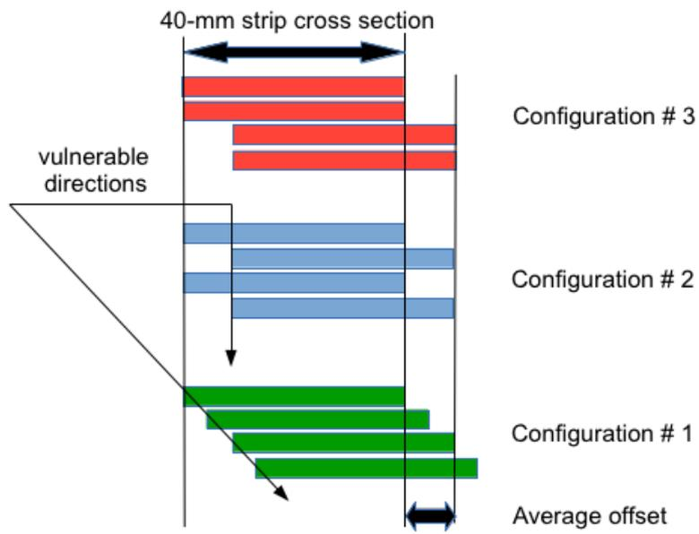
Figure 2. Strip layouts implemented in the simulation.
