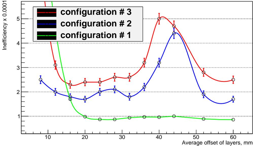
Figure 7. The muon registration inefficiency for a stack of four layers for the three configurations described in the beginning of the section 2. Notice that the offset of the second layer in the first configuration is a half of the *average offset*.
