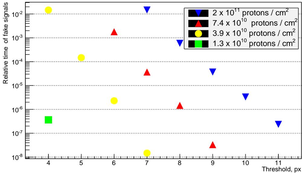
Figure 10. The fraction of time lost due to fake muon signals caused by coincident noise signals of MPPC vs. the readout threshold for four irradiation doses of MPPCs:  $1.3 \cdot 10^{10}$  p/cm<sup>2</sup>,  $3.9 \cdot 10^{10}$  p/cm<sup>2</sup>,  $7.4 \cdot 10^{10}$  p/cm<sup>2</sup>, and  $2 \cdot 10^{11}$  p/cm<sup>2</sup> (based on [2]). The length of the veto window is taken to be 100 ns, the signal resolution time of the veto counter being 20 ns.
