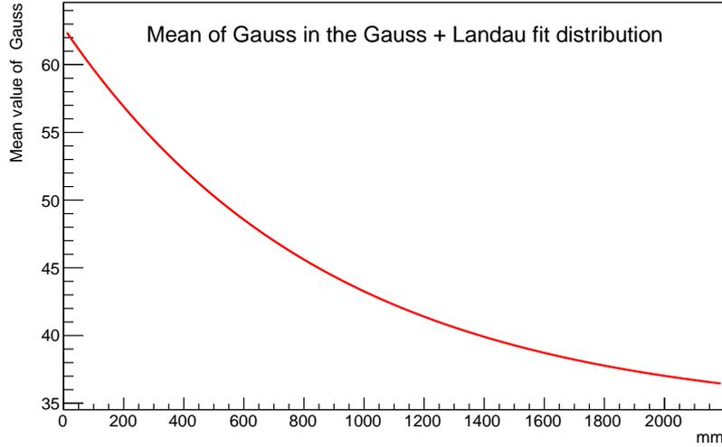
Figure 4. Variation of a fit parameter of spectra along a 2218 mm strip.
