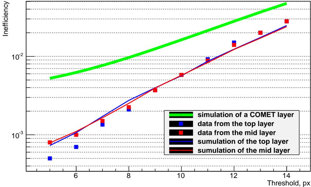
Figure 6. Results of simulation for COMET single layer and for inefficiency measurement for both top and middle layers described in [3].
