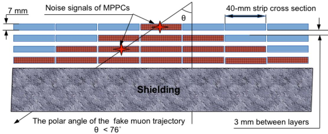
Figure 9. The minimal scheme of strips that should be examined for a coincident noise signal.
