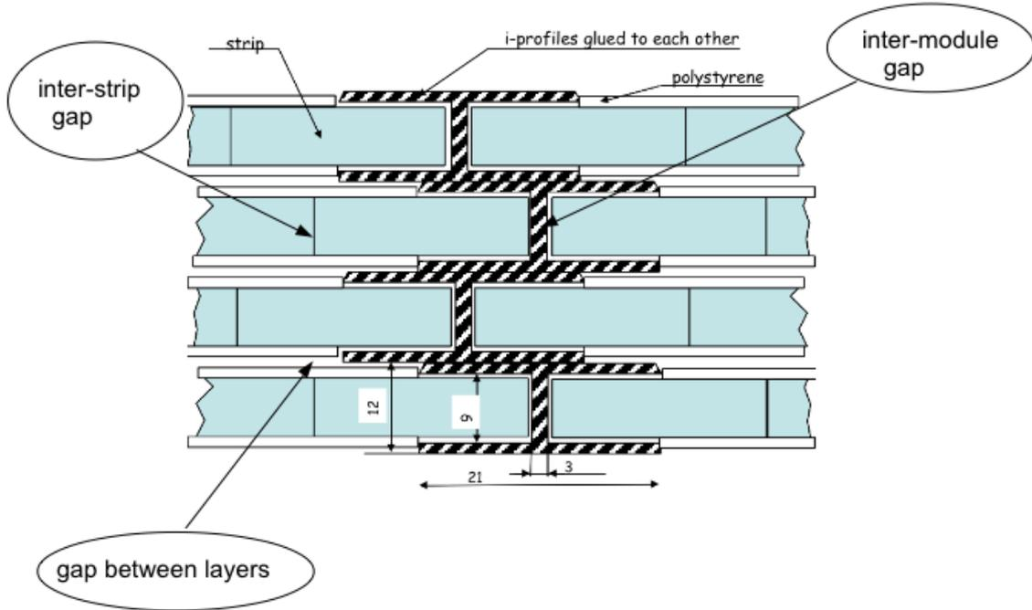
Figure 1. One of possible layouts of strips.
