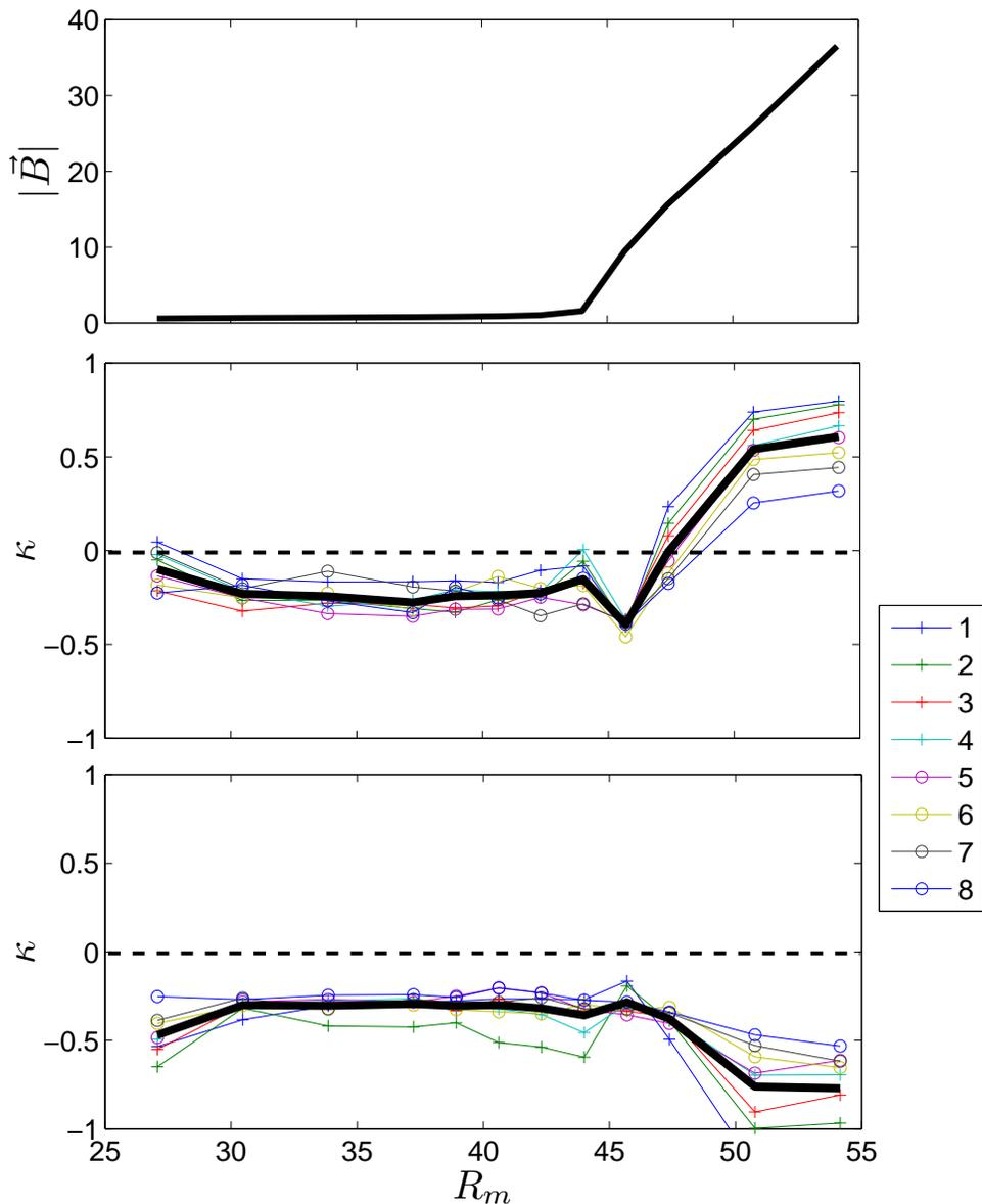
FIG. 4. Upper panel: bifurcation in terms of the magnetic field averaged over all the sensors. Central panel: Shape parameters vs Reynolds magnetic number for the 8 group of sensors (each in a different color),  $\langle \kappa \rangle$ , (thick black line) and Gumbel law  $\kappa = 0$  (dashed line) in the R configuration. Lower panel: same as the central panel but for the minima.
