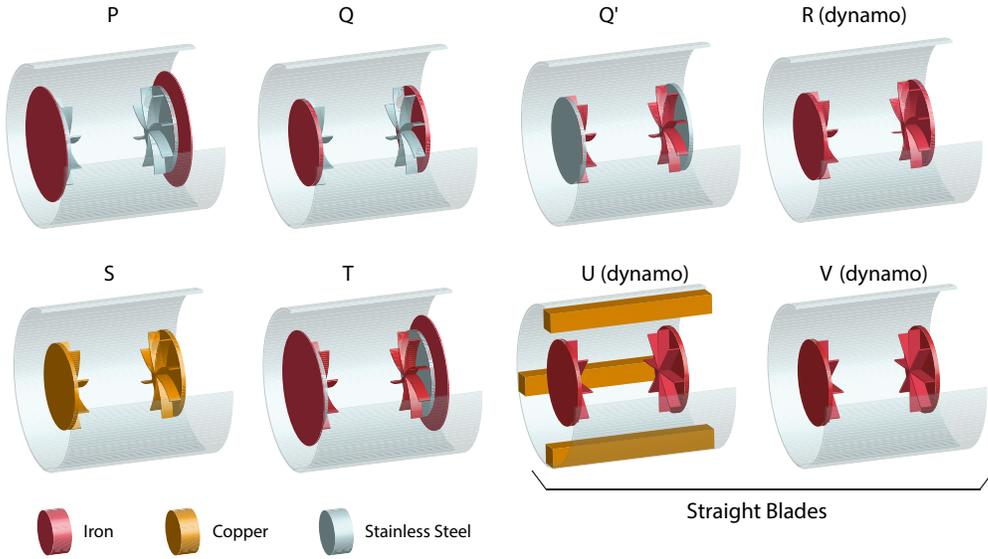
FIG. 2. Schematic representation of the studied VKS configurations. Gray colors stands for stainless steel, yellow color for copper and red for soft iron.
