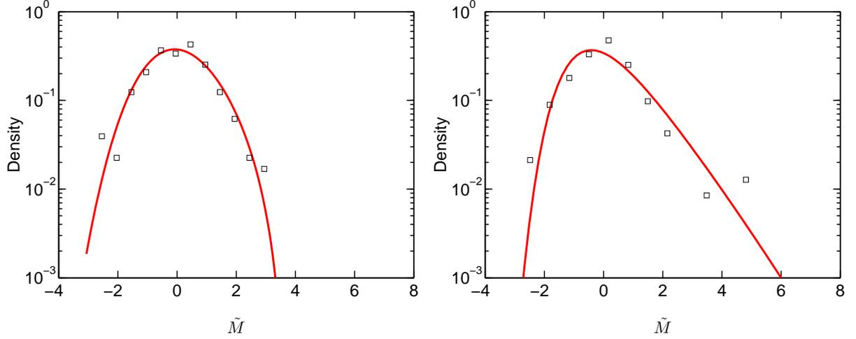
FIG. 5. Two histograms for the normalized maxima  $\tilde{M}$  of the sensors 6 (black markers) and correspondent fits to the GEV distribution (red lines). Left:  $Rm \simeq 27$  the maxima are bounded:  $\kappa = -0.21$ . Right:  $Rm \simeq 48$ , some maxima are detached with respect to the bulk statistics. These events trigger the transition of  $\kappa$  towards positive values:  $\kappa = +0.01$ .
