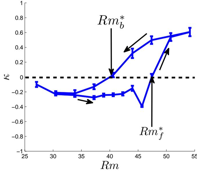
FIG. 6.  $\langle \kappa \rangle_l$ , (blue line) and Gumbel law  $\kappa = 0$  (dashed black line) vs magnetic Reynolds number in the R configuration. The arrows indicate the direction of variation of  $Rm$  in the experiment.
