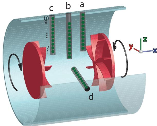
FIG. 1. Experimental setup, showing the location of the Hall probes.  $x$  is the axial coordinate directed from impeller 1 to impeller 2
