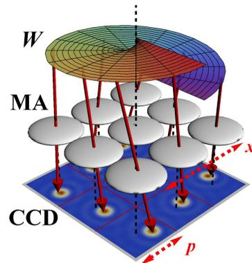
FIG. 1. **The principle of the SH wavefront sensor.** A microlens array (MA) subdivides the wavefront ( $W$ ) into multiple beams that are focused in a CCD camera. Local slope of the wavefront over each microlens aperture determines the location of the spot on the CCD. Red arrows represent normals to the wavefront.
