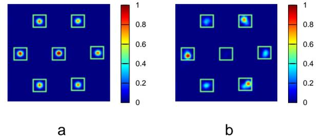
FIG. 3. **Experimental CCD signal.** Rescaled 8-bit data corresponding to 7 microlenses placed in a hexagonal geometry,  $81 \times 81$ -pixels region, is displayed in both panels. a) Data of the plane wave used for calibration; b) data of the partially coherent vortex beam in Eq. (5). Green squares enclose the data used for the reconstruction. The intensity from the central microlens vanishes due to the presence of a phase singularity.
