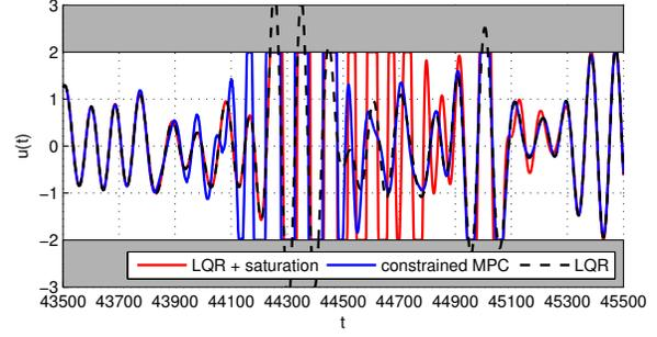
Fig. 13. Control design in presence of constraints: the grey regions indicate the limits imposed to the amplitude of the control signal  $u(t)$ . The control  $u(t)$  is designed following two different strategies: LQR with a saturation function (—) and constrained MPC (—), see §3.2.2. The LQR solution (---) is introduced as reference. The performances of the controllers are shown in terms of *rms*-velocity reduction in Fig. 14.
