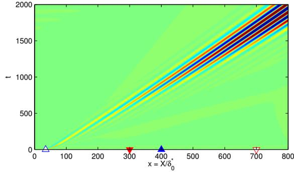
Fig. 2. Response to a small, localized initial condition in a Blasius boundary-layer flow. A Tollmien-Schlichting wave-packet emerges and grows exponentially while propagating downstream. Contours of the streamwise component of the velocity are shown as a function of the streamwise direction ( $x$ ) and time ( $t$ ). The location along the normal-direction  $y$  is chosen in the vicinity of the wall.
