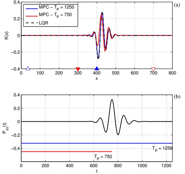
Fig. 15. In (a) the LQR solution (§3.1.1) is compared to the MPC gains computed for two different times of optimization  $T_p$  without constraints, see §3.2.3. The optimization times are compared to the impulse response  $\mathcal{P}_{zu}(t)$  (b). Note that for longer time  $T_p$ , covering the main dynamics of the impulse response  $\mathcal{P}_{zu}(t)$ , the MPC and LQR solutions are equivalent.
