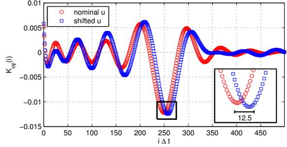
Fig. 24. Robustness to uncertainties of the system: FXLMS control gain  $\tilde{\mathcal{K}}_{uy}(i)$  ( $\square$ ) is shifted along the time-discrete coordinate if compared to the static LQG gain ( $\circ$ ) to compensate for the un-modelled shift in actuator position. [script10.m]
