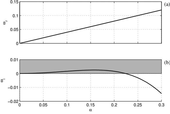
Fig. 3. The real frequency  $\omega_r$  and its imaginary part  $\omega_i$  are shown as a function of the spatial frequency  $\alpha$ , in (a) and (b), respectively. The relation among the spatial and temporal frequencies is given by the dispersion relation (8). Positive values of  $\omega_i$  characterize unstable waves (grey region).
