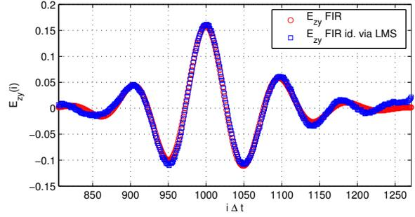
Fig. 18. Impulse responses ( $y \rightarrow z$ ) of the estimator as a function of the discrete-time. Red circles ( $\circ$ ) correspond to the FIR time-discrete Kalman-filter-based kernel  $\tilde{\mathcal{E}}_{zy}(i)$  and the blue squares ( $\square$ ) to the one identified by the LMS algorithm. [script07.m]
