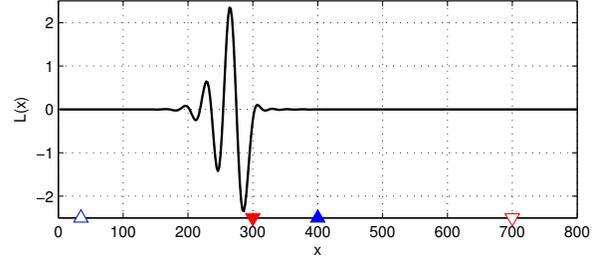
Fig. 16. Kalman estimation gain  $\mathbf{L}$  computed for  $R_d = 1$  and  $R_n = 0.1$ , (see §4.1.1). [script06.m]
