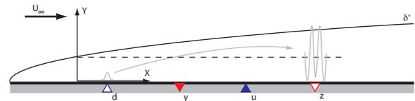
Fig. 1. Scheme of a Blasius boundary-layer flow developing over a flat plate. A disturbance modelled by  $d$  grows exponentially while convected downstream. The actuator  $u$  is used to attenuate the disturbance before it triggers transition to turbulence; the actuation signal is computed based on the measurements provided by the sensor  $y$ . The output  $z$ , located downstream of the actuator, estimates the efficiency of the control action.
