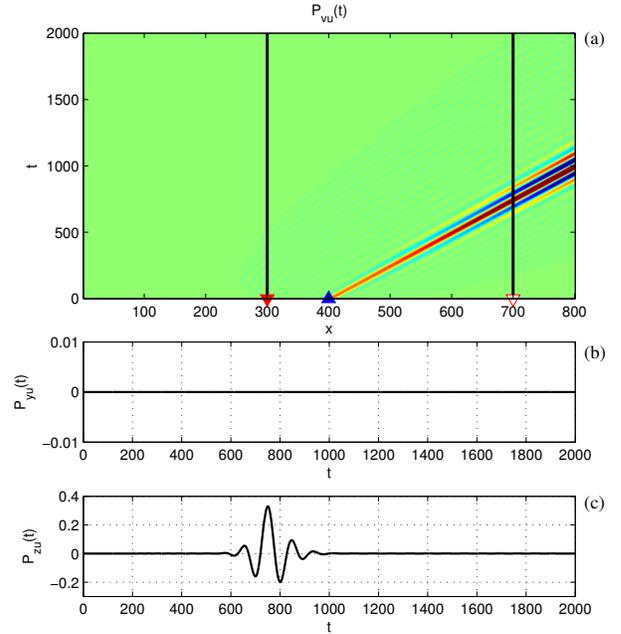
Fig. 10. The disturbance generated by the impulse response of the system at the actuator location  $u$  in (a) is shown as a function of the streamwise direction ( $x$ ) and time ( $t$ ). The wave-packet is detected only by the output  $z$  (c); due to the convective nature of the flow, the sensor placed upstream of the actuator can not detect the propagating disturbance, and the resulting signal is practically null (b). [script02.m]
