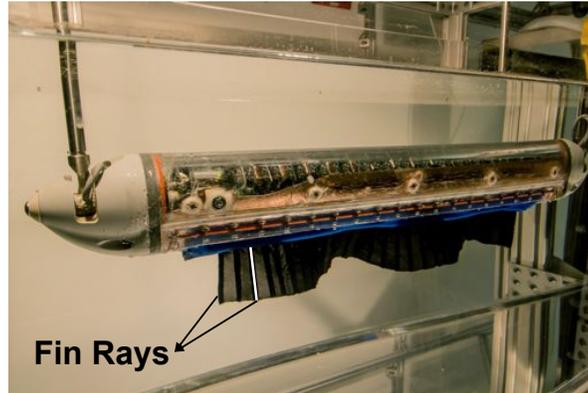
**Figure 10.** The robotic knife-fish used in the drag-thrust decomposition experiments. The robotic ribbon-fin is composed of 32 fin rays and a Lycra fabric connecting the rays. One of the fin rays is coloured white to highlight it.
