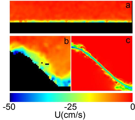
**Figure 9.** A comparison between the boundary layer due to, a) flow past a flat plate, b) slithering motion of a robotic ribbon fin, c) and slithering motion of a modeled robotic fin in a simulation. The boundary layer is shown on a horizontal plane 1 cm above the bottom edge of the fin toward the robot body. The color bar represents the axial velocity.
