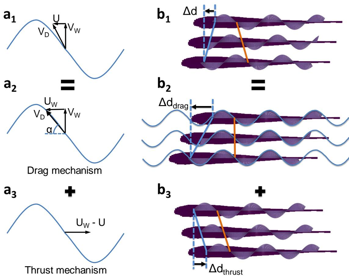
**Figure 2.** a) The proposed kinematic decomposition into drag and thrust producing mechanisms. The front end is on the left. b) The kinematic decomposition applied to a modeled black ghost knifefish. Each row, from top to bottom in each of the undecomposed, drag, and thrust mechanism, is at increasing instants of time.
