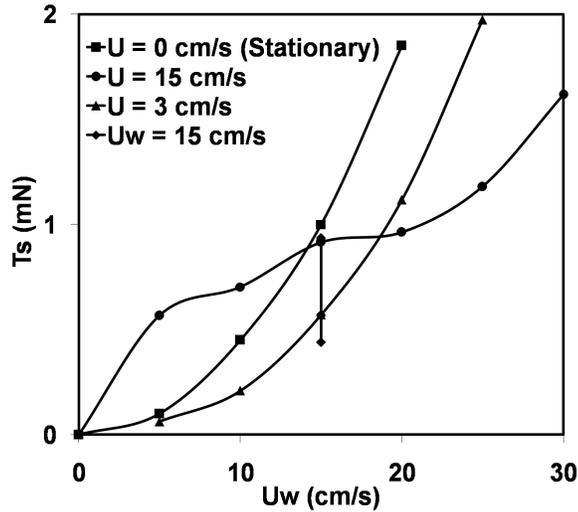
**Figure 7.** The thrust force  $T_s$  computed as a function of  $U_w$  for each data point in Fig. 2 by assuming a decomposition according to equation 2. In this case the data do not cluster along a single curve. The legend identifies different simulation sets. For example, the set with  $U_w = 15$  cm/s was the one where  $U_w$  was fixed and the value of  $U$  was changed.
