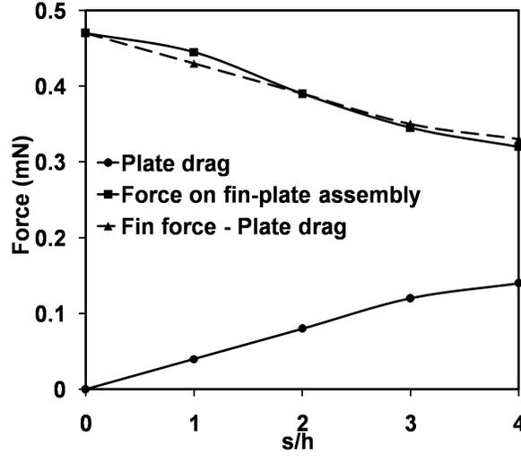
**Figure 13.** Force  $F_p$  on the plate (—●—), force  $F_{fp}$  on the fin-plate assembly (—■—), and  $F_f - F_p$  (—▲—) as a function of  $s/h$ . Agreement between  $F_{fp}$  and  $F_f - F_p$  shows that there is no momentum enhancement.
