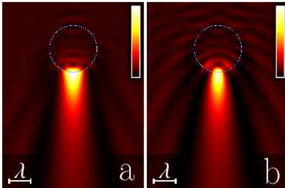
Figure 1: Near-field intensity distributions of the total wavefield in (a) the  $x - z$  plane and (b) the  $y - z$  plane for the LG beam with  $m_{\text{LG}} = 0$ ,  $f = 0.05$  and  $|\mathbf{R}_d| = 0$ . The parameters are:  $R_p = \lambda$  is the scatterer radius and  $n_p = 1.3$  ( $n_m = 1.0$ ) is the refractive index inside (outside) the particle.
