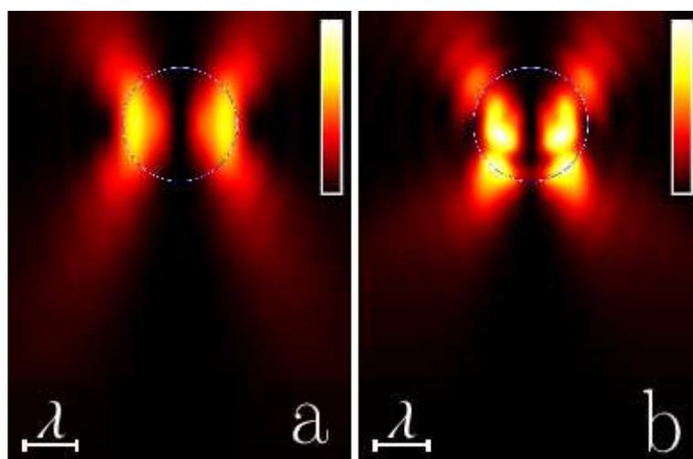
Figure 3: Near-field intensity distribution in the  $x - z$  plane of (a) the incident wave beam and (b) the total wave field for the LG beam with  $m_{\text{LG}} = 2$ ,  $f = 0.25$  and  $|\mathbf{R}_d| = 0$ .
