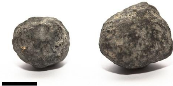
Fig. 1. Two fragments of Khameneh alleged meteorites weighing 6 and 11 grams, on the left and right side, respectively. Scale bar: 10mm
