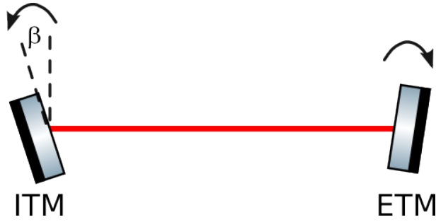
Figure 2: Sign convention for misalignment angles. The illustration shows a misalignment of the ITM and ETM by a positive numerical value of the misalignment angle.
