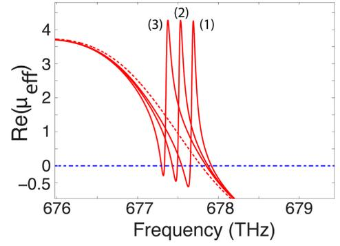
FIG. 5. (Color online) Tunability of the MNP-QD nanoring metamaterial. The real part of  $\mu_{eff}$  for different MNP-QD detunings. We plot: (1)  $\Delta = 0.195$ , (2)  $\Delta = 0.196$ , and (3)  $\Delta = 0.197$ . All detunings are in units of  $10^{15}$  rad  $s^{-1}$ . The dashed line shows the bare MNP nanoring in the absence of QDs.
