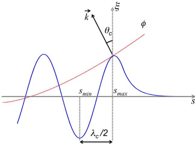
FIG. 7. (Color online) Schematic of the behavior of an Airy beam: When the wavevector  $\vec{k}$  of the Airy beam, which is normal to the wavefront  $\phi$ , reaches the maximum paraxial value  $\theta_c = \frac{\pi}{6}$  the oscillations in the profile must dampen in order to remain physical. At that point, the distance between two extreme points in the profile must be of the order of half the critical wavelength  $\lambda_c$ .
