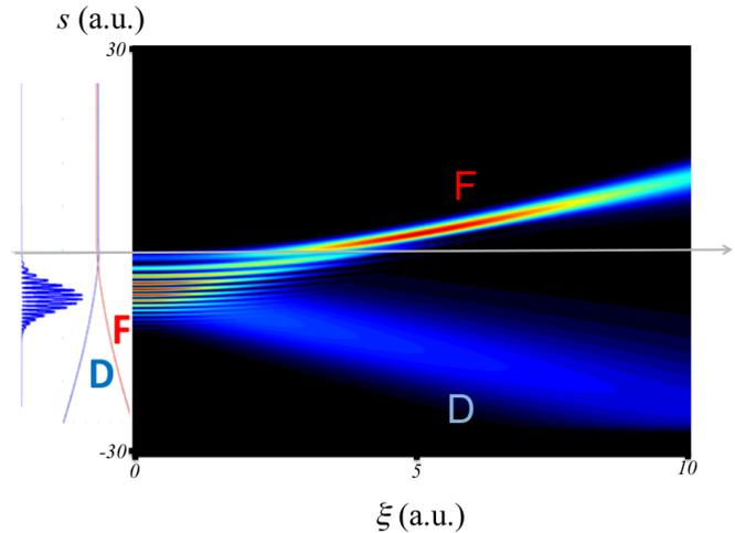
FIG. 6. (Color online) Propagation of off-axis Airy-Gauss beam using arbitrary dimensionless units
