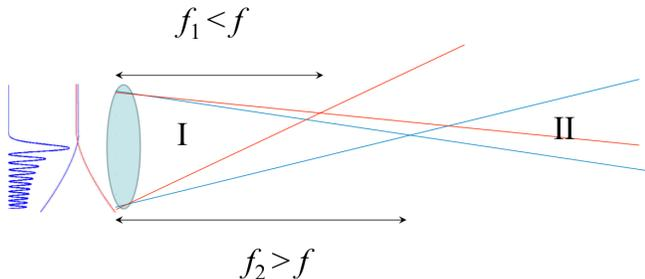
FIG. 5. Schematic ray tracing of the double focusing of an Airy beam related to that shown in Figure 4.
