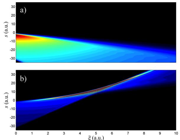
FIG. 2. (Color online) Behaviour of the independent propagation of the  $\text{Ai}H^{(1)}$ , a), and of the  $\text{Ai}H^{(2)}$ , b), component of the Airy beam in arbitrary dimensionless units.
