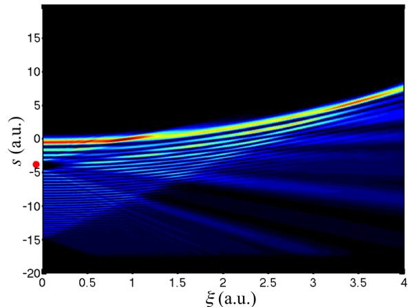
FIG. 3. (Color online) Propagation of an obstructed Airy beam (in arbitrary dimensionless units) showing self-healing. Notice the presence of two shadows. The red dot at the edge of the figure indicates the position where the obstruction has been located.
