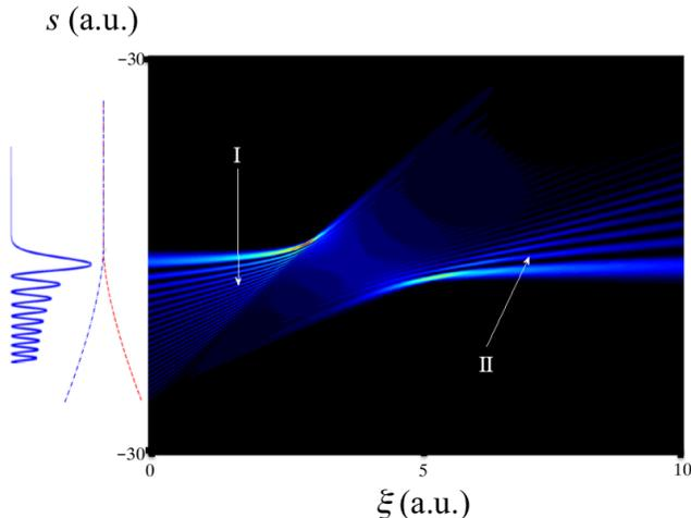
FIG. 4. (Color online) Behaviour of a focussed Airy beam (in arbitrary dimensionless units), observe the two regions due to the focusing of the two Hankel travelling waves. In the edge of the figure we have indicated the profile of the Airy beam as well as the two wavefronts of the beam.
