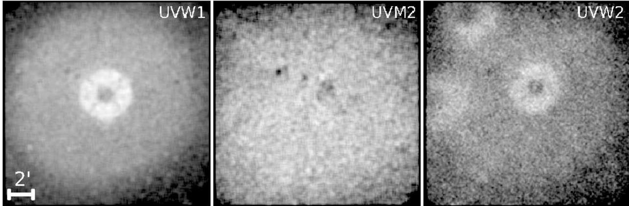
**Figure 2.** Images of the persistent scattered-light artifacts in the UVOT filters. The images were generated by stacking many deep exposures after removing point sources and processing up through flat-fielding and exposure correction, and are in detector coordinates. The final images have been lightly smoothed. Each of the visible rings has an outer radius of 2 arcmin.
