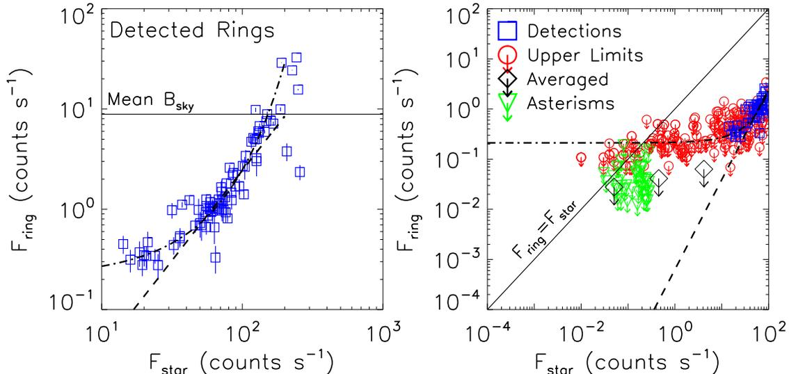
**Figure 6.** *Left:* Instrumental scattered light flux ( $F_{\text{ring}}$ ) as a function of the incident flux of the associated star ( $F_{\text{star}}$ ) for the *Swift wvm2* filter. The best exponential and log-linear models have been overplotted. *Right:*  $F_{\text{ring}}$  detections and limits at lower  $F_{\text{star}}$ , including limits from averaged data. See Section 3 for discussion.
