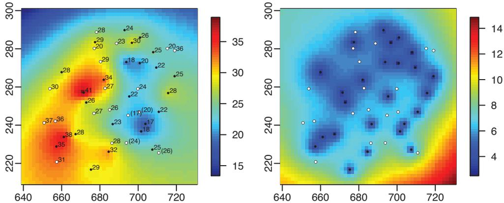
**Fig. 3:** Conditional simulation of extreme rainfall over the region of Zürich for 1 June 1962. Left: mean of the conditional simulation of daily cumulative rainfall (in mm). Black dots correspond to the locations on which we conditioned, white dots to the data used for validation with their observed values (written in parentheses under the thresholds). Right: standard deviation for the conditional simulation.
