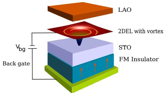
FIG. 6. (Color online) Schematic picture of the proposed setup for realization of MBS in  $\text{LaAlO}_3/\text{SrTiO}_3$  interface.
