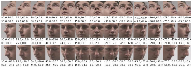
Fig. 3. Some estimation results of the second sequence of person 13. The top numbers are the ground truth yaw and pitch and the bottom numbers are the estimated yaw and pitch.
