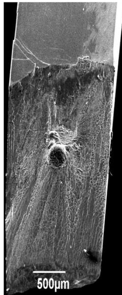
**Figure S7** | A scanning electron micrograph of the fracture surface. Several shear bands are seen adjacent to the fracture surface. A 300 µm diameter pore due to a casting defect is visible.
