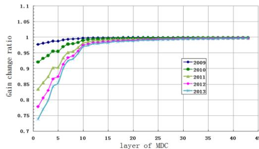
Figure 8: Gain drop of the chamber
