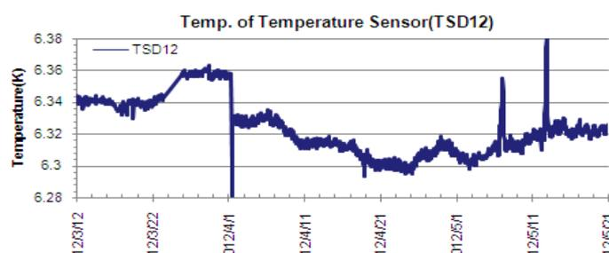
Figure 31: Temperature of current leads transition section
