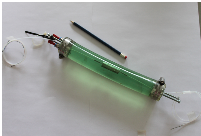
Figure 4. Sensor located in an oil filled hose.
