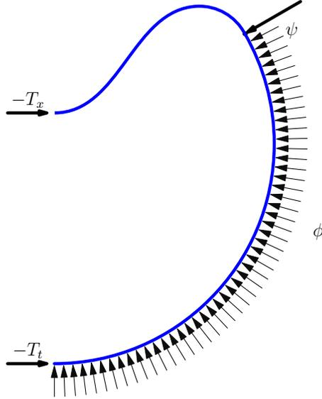
Figure 7: Internal and external forces acting on the half-beam in case of unilateral and frictionless contact. The forces  $T_x$  and  $T_t$ , as given in equations (45) and (46) respectively, are negative, so that the beam is under compression for any admissible configuration. The concentrated force  $\psi$  is necessary to balance the vertical components of the internal forces at  $s = \bar{s}$ .
