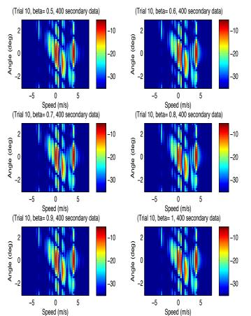
Fig. 7.  $\log_{10}(\widehat{\Lambda}_{SCM-DL})$  for different values of  $\beta$ : angle/speed map with parameters m = 256, N = 400. The colour scale is in dB with a dynamic of 30 dB from the maximum value of  $\log_{10}(\widehat{\Lambda}_{SCM})$
