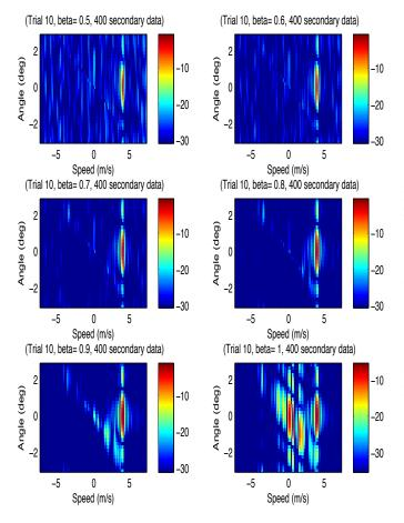
Fig. 5.  $\log_{10}(\widehat{\Lambda}_{S-FPE})$  for different values of  $\beta$ : angle/speed map with parameters m = 256, N = 400. The colour scale is in dB with a dynamic of 30 dB from the maximum value of  $\log_{10}(\widehat{\Lambda}_{S-FPE})$
