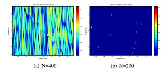
Fig. 11.  $\log_{10}(\widehat{\Lambda}_{SCM})$ : angle/speed map with parameters m = 256 for the range bin 268 and for different values of N. The colour scale is in dB with a dynamic of 30 dB from the maximum value of  $\log_{10}(\widehat{\Lambda}_{SCM})$
