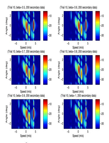
Fig. 9.  $\log_{10}(\widehat{\Lambda}_{S-FPE-W})$  for different values of  $\beta$ : angle/speed map with parameters m = 256, N = 200. The colour scale is in dB with a dynamic of 30 dB from the maximum value of  $\log_{10}(\widehat{\Lambda}_{S-FPE-W})$
