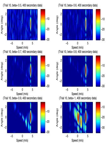
Fig. 6.  $\log_{10}(\widehat{\Lambda}_{S-FPE-W})$  for different values of  $\beta$ : angle/speed map with parameters m = 256, N = 400. The colour scale is in dB with a dynamic of 30 dB from the maximum value of  $\log_{10}(\widehat{\Lambda}_{S-FPE-W})$
