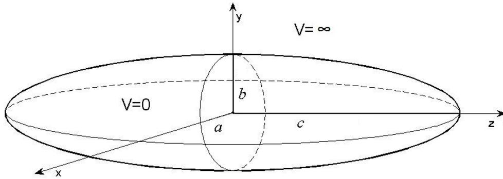
**Fig.1** Nanorod of ellipsoidal shape with major semi-axis  $c$  (the nanorod axis) much larger than minor semi-axes  $a = b$ .
