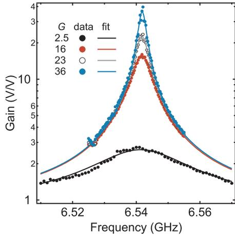
FIG. S6: JPA small-signal amplitude gain at different bias points. The values of  $G$  are obtained by fitting  $|G_{s,\Delta}|$  to each curve using Eq. (S3). The other fit parameter is  $\kappa_e/2\pi = 83, 91, 92$  and  $91 \pm 1$  MHz for  $G = 2.5, 16, 23$  and  $36$ , respectively. As expected,  $\kappa_e \approx \mathcal{G}\kappa_{\text{JPA}}$  is approximately constant for  $G \gg 1$ .
