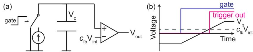
FIG. S5: Voltage-controlled delayed trigger. (a) Simplified diagram of the homemade circuit. A current source, switched by a marker bit from the AWG5014, ramps a voltage  $V_c$  linearly from  $-2$  to  $2$  V in 200 ns. This voltage is compared to the signal from the FPGA,  $c_{\text{fb}} V_{\text{int}}$ . (b) The output trigger is generated when  $V_c$  crosses  $c_{\text{fb}} V_{\text{int}}$ .
