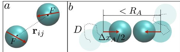
FIG. 1: a) Self-propelled (SP) particles (with propulsion force  $F$ ) interacting via a Lennard–Jones potential. b) Self-displacing (SD) particles moving towards each other over a distance  $\Delta x_A$  with a rate  $\nu$  if they are within a distance  $R_A$ . Particles also undergo diffusion ( $D$ ). Depending on the values of  $\Delta x_A$ ,  $\nu$  and  $D$ , either clustering or collisions dominates.
