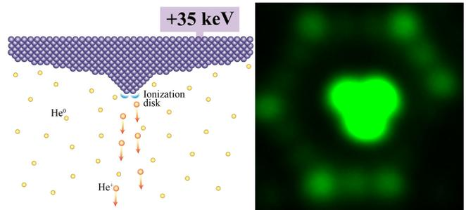
Figure 1. (Color online) (a) Sketch of a GFIS. Ionization happens dominantly at the most protruding corner and edge atoms. (b) Actual SFIM image of a GFIS. The center trimer and the edges and corners of the next crystal plane are visible.
