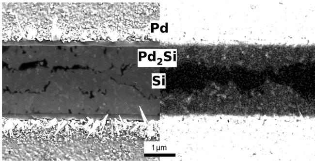
Figure 7. Subsurface imaging in HIM. (a) Surface sensitive SE image obtained from SiO<sub>2</sub> covered Pd<sub>2</sub>Si interconnects. (b) Simultaneously recorded BSHe image showing the Pd deposits (bright, top and bottom) and the buried Pd<sub>2</sub>Si layer. The shape of the two Pd diffusion fronts is clearly discernible between the two Pd contacts.
