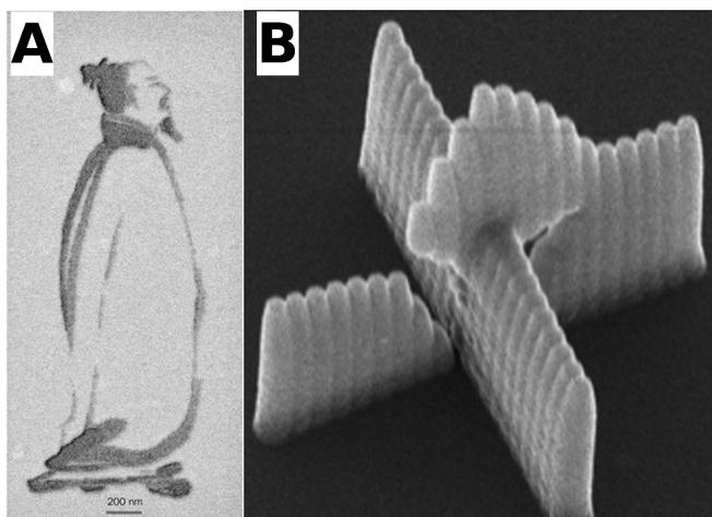
Figure 11. Examples of structures created using He beam induced metal deposition. (A) 100,000 $\times$  demagnified copy of a 13th century painting of the Chinese poet Li Bai. (B) Stacked cross formed by exploiting shadowing of the precursor gas (FOV: 1 $\mu$ m). Adapted with permission from Scanning 34, 90–100 (2012). Copyright 2012 Wiley Periodicals, Inc.
