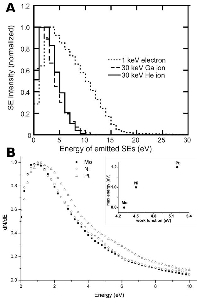
Figure 3. SE yield in HIM. (A) Comparison of calculated SE yields for electrons, Ga ions and He ions. Reproduced with permission from [38]. (B) Experimentally obtained SE yield for three different metals. The dependence of the peak position on work function is shown as an inset. Reproduced with permission from Proc. SPIE, Vol. 8036, 80360O-1–80360O-10 (2011). Copyright (2011) SPIE.
