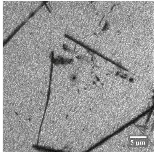
Figure 8. (IL image of a GaN surface. He<sup>+</sup> beam energy is 35 keV. FOV: 45 μm
