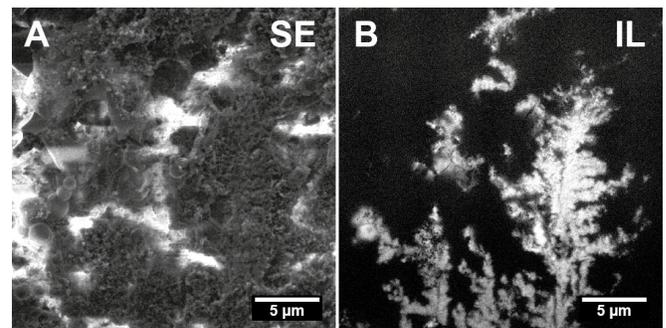
Figure 9. Simultaneously recorded SE and IL images of NaCl residues from water solution on a metal. IL images reveal a distribution of NaCl. He<sup>+</sup> beam energy is 35 keV. FOV: 25 μm
